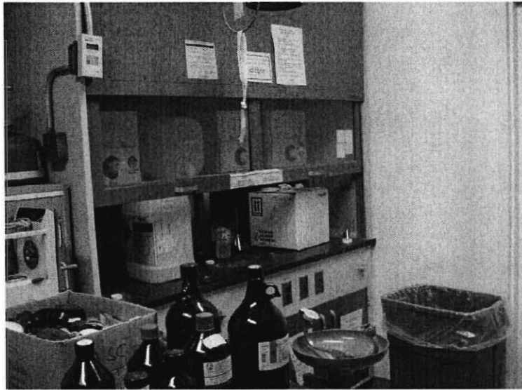
Figure 35 - Fume hood in stockroom, eyewash at bottom
