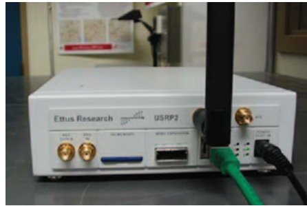
(a) Front view of a Universal Software Radio Peripheral – Version 2 (USRP2) software-defined radio platform by Ettus Research LLC.
