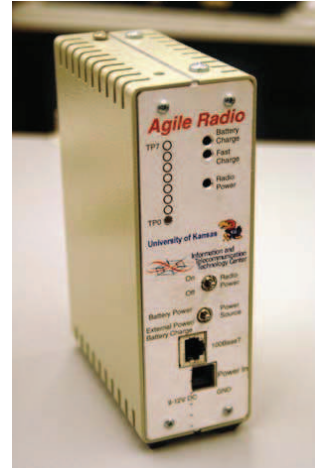
(b) Front view of a Kansas University Agile Radio (KUAR) software-defined radio platform.
