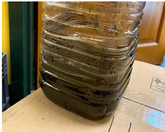
Figure 10. Results from density separation of a wet soil sample.
