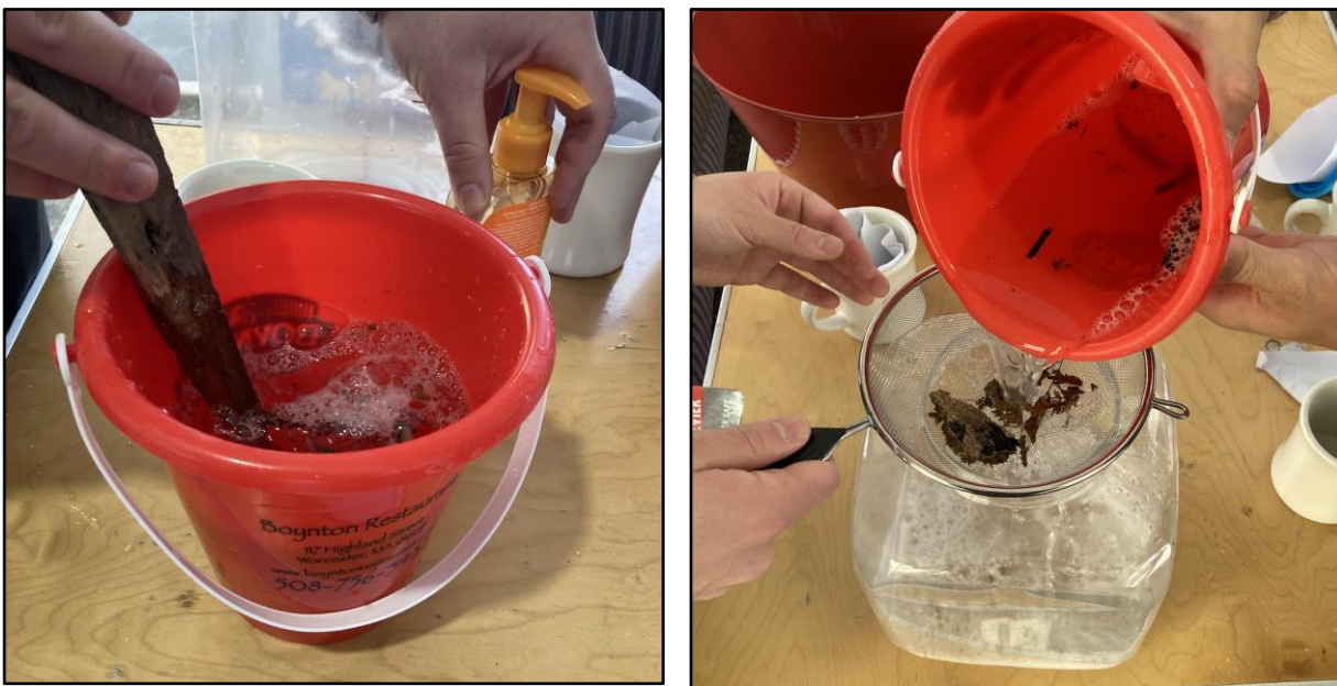
Figure 8. The first image shows us preparing a contaminated sample of water using face wash with microbeads. The second is the filtration process of the contaminated sample using a large kitchen strainer.
