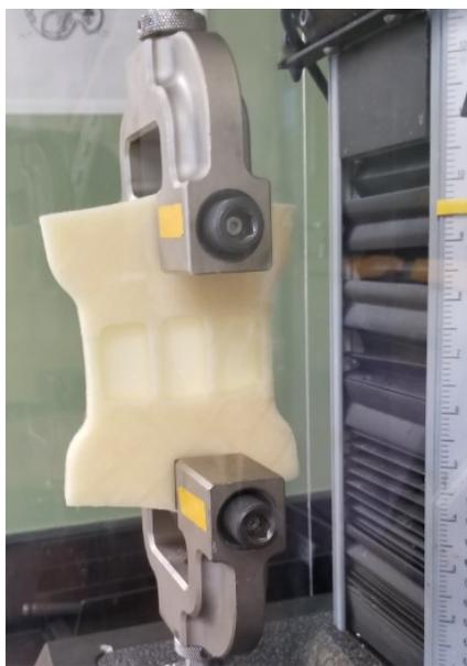
Figure 31. Tensile stretch of “Butterfly Squares” well plate
