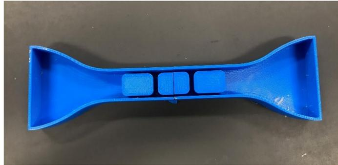
Figure 37. ABS well plate mold
