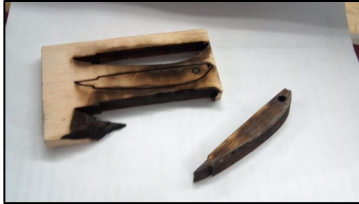
Figure 30: Burnt Balsa Wood
