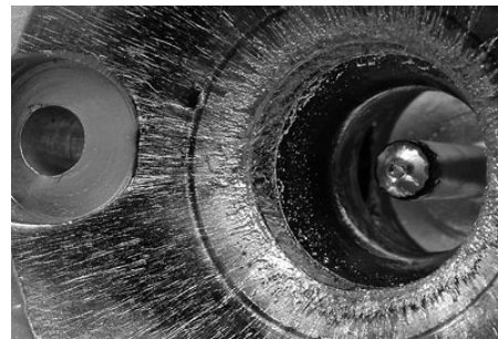
Figure 70: Anode Material Loss
