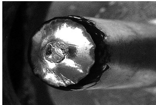
Figure 68: Cathode Spot at Tip
