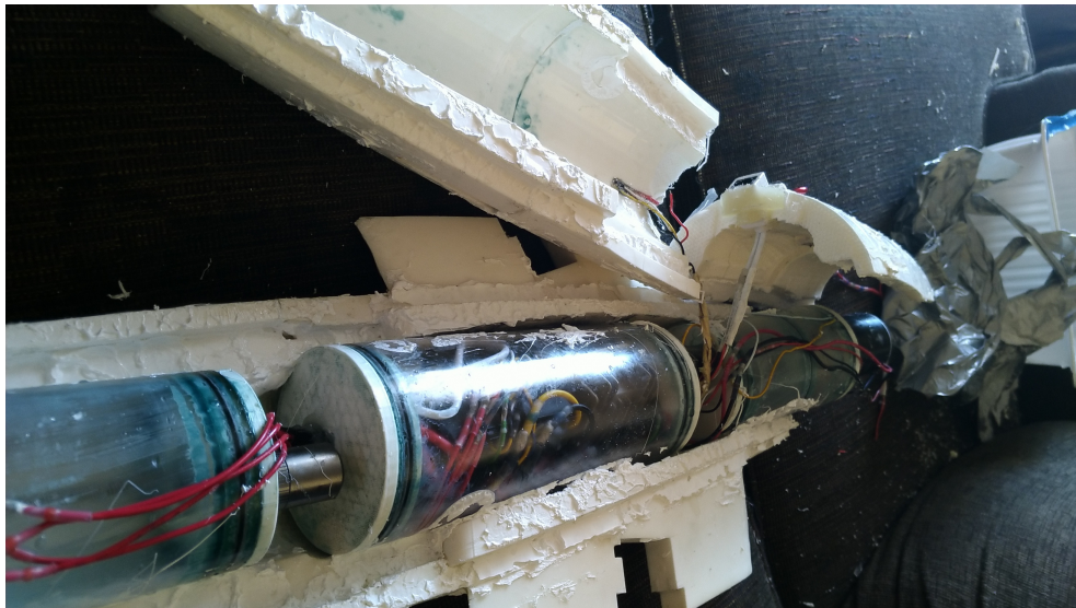
Figure 47: Upon opening the craft, the top broke in two.
