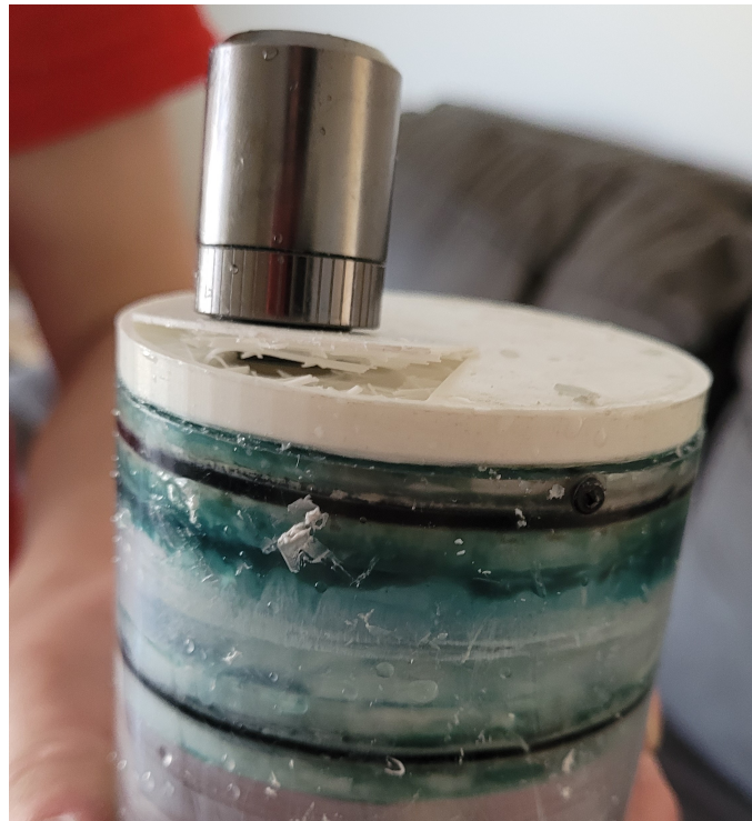
Figure 53: The broken front endcap on the rear ballast
