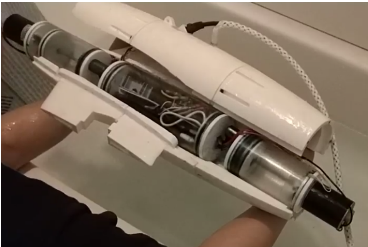
Figure 41: Bathtub testing of the craft for the semi-submersion test
