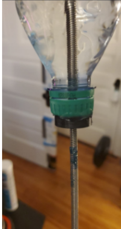
Figure 18: Test for leakage through leadscrew flange combination
