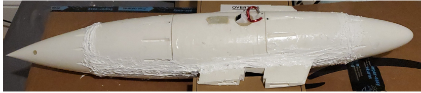
Figure 44: Letting the silicone rest for 24 hours before the first test
