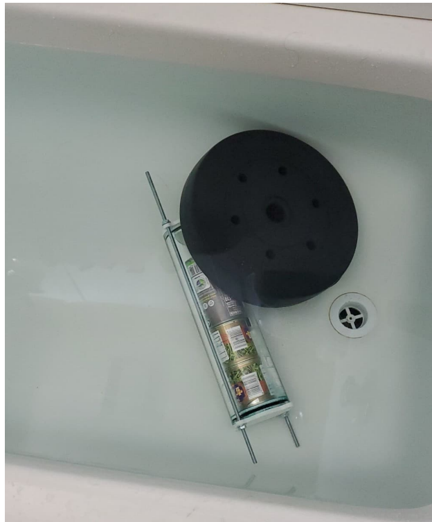
Figure 40: Pressure hull submersion test
