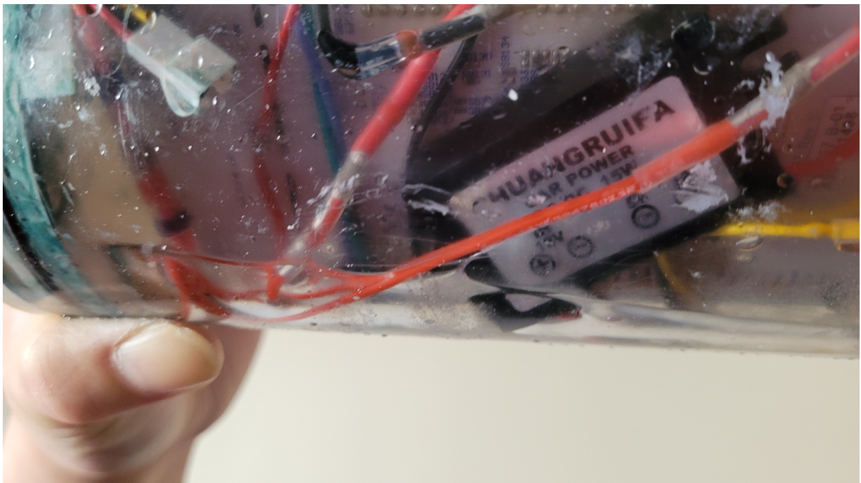
Figure 52: A few millimeters of water leaked into the pressure hull.
