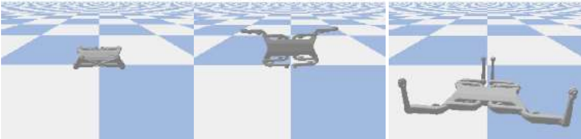
Figure 45. The agent trying to stand quadrupedally using (23) as the reward function. The agent tended to “jump” up at the beginning to achieve the height reward but ends up tipping over onto its back—achieving a perfect “flat” reward. Near the end of the episode, the agent tries to move its legs to lift it up, but that is not enough to achieve quadrupedal standing.
