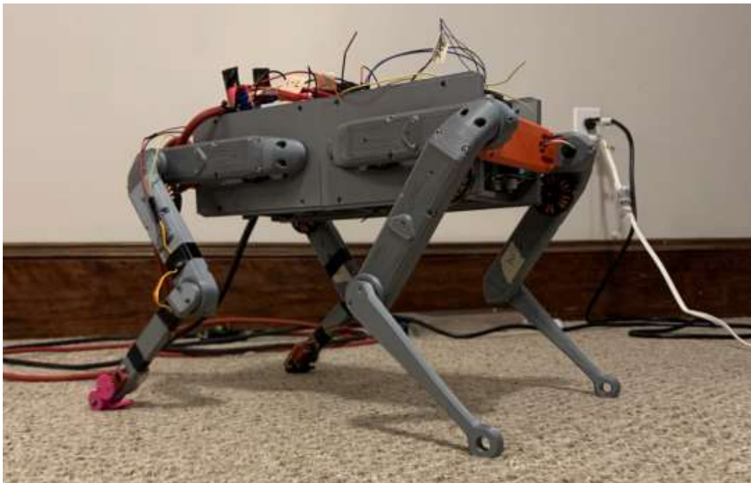
Figure 33: Robot standing after reducing the weight of wiring and implementing the new leg configuration.
