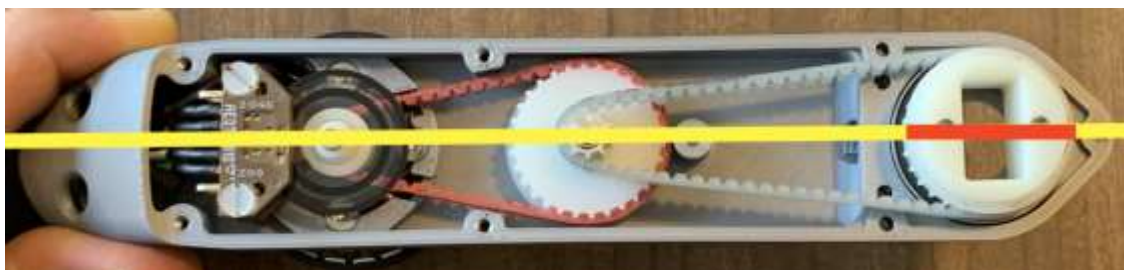
Figure 25: Hip module’s horizontal axis (yellow line) aligned with the pulley’s horizontal axis (red line)
