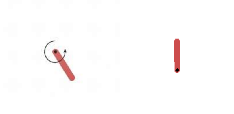
Figure 17. Open AI Gym's Pendulum-v0 environment. Here, the agent applies torques to a pendulum with one rotational point. On the left, the agent's torque is being visualized by an arrow representing direction and magnitude. On the right is a properly trained agent. This agent is actually applying torques to balance the pendulum, but they are so minute that it is not visible in the screenshots.
