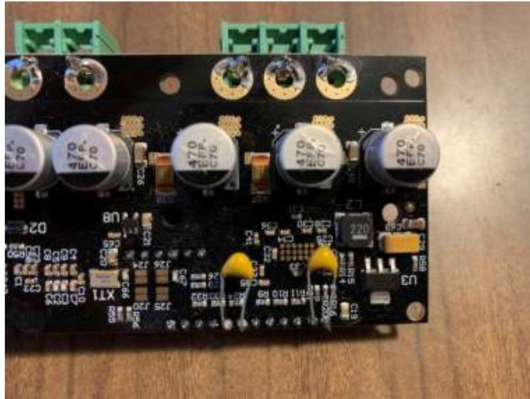
Figure 22: 47nF capacitors soldered to both ODrive axes
