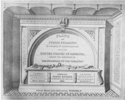
Figure 12: Plans of Public Buildings Under Construction under the supervision of Architect of the Treasury Ammi B. Young, 1856. Notice the I-beam and brick arch floors detailed on the top of the image.
