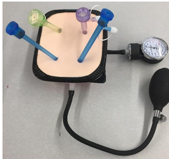
Figure 6.1. Leak Test Setup.
