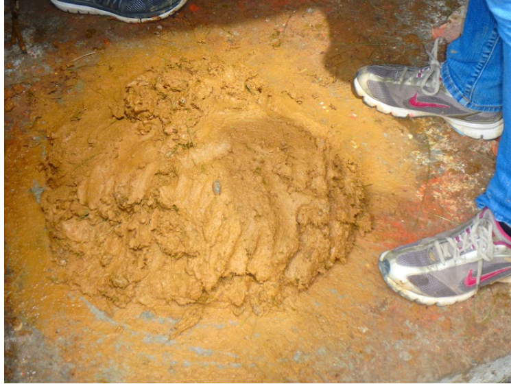
Figure 17. Cow dung, dirt, pine needles, and water mixture (Baker, 2016)
