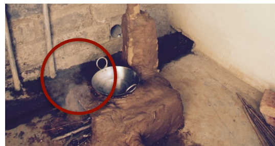
Figure 10. Smoke leaving from front opening during testing; side pipe covered (Zhang, 2016)
