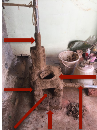
Figure 9. Comparison of traditional stove in Nehri Village to second prototype. Arrows note the changes made, which include a box-shaped stove, a closeable front opening, a top and side pipe, a closed stovetop, and a baseplate. (Zhang, 2016)
