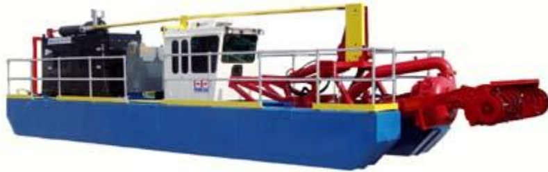
Figure 5.7: Mud Cat Dredge (Mud Cat Dredges, 2010)
