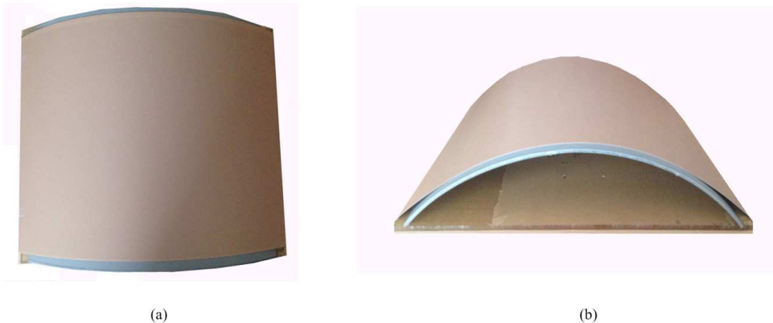
Fig. 3-3. The physical scan surface (PSS): (a) top view; (b) side view
