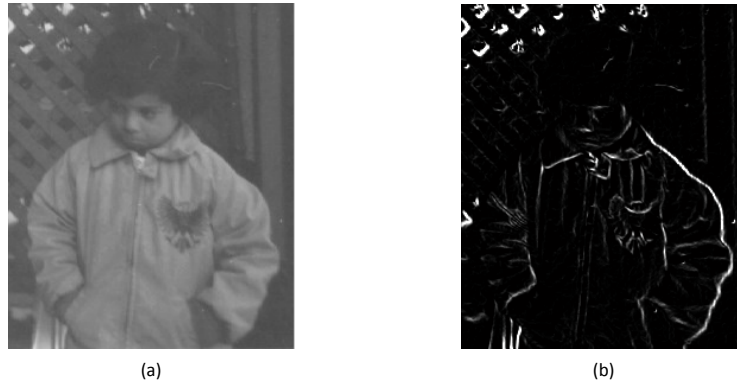
Figure 2.40: Illustration of Sobel filter
