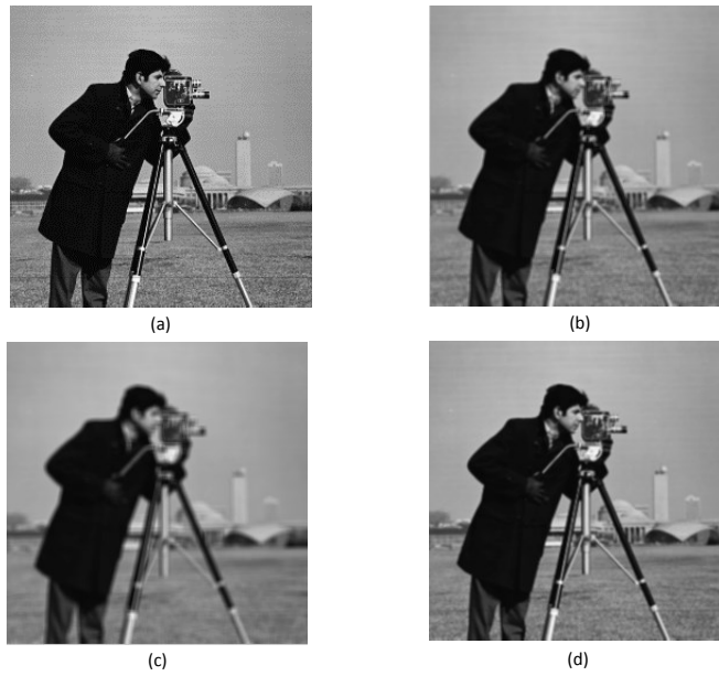
Figure 2.26: Illustration of 2D FIR filter
