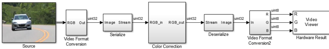
Figure 2.4: Flow chart of color correction system in Simulink
