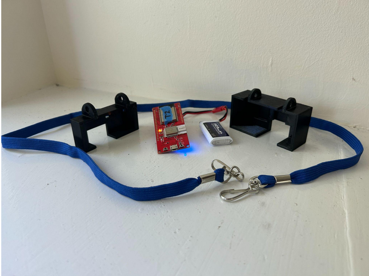
Figure 38: Disassembled UWB Tag
