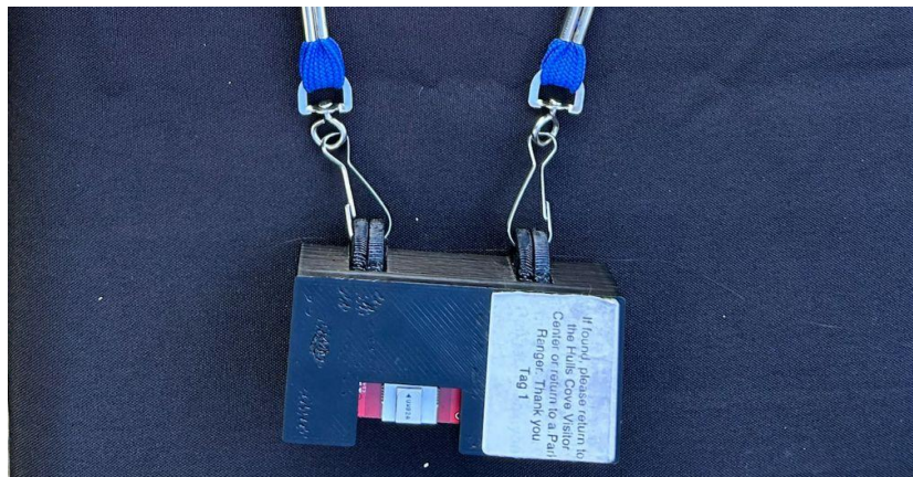
Figure 6: Ultrawideband Tracking Tag Attached to a Lanyard
