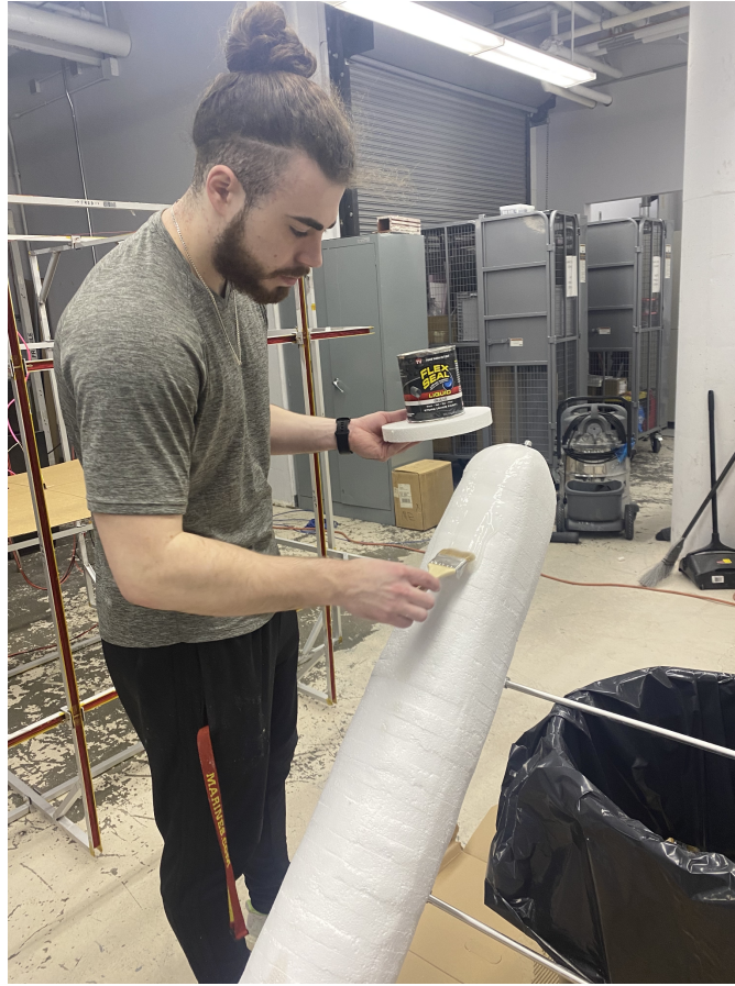
Figure 25: Flex Seal Application to the Hull
