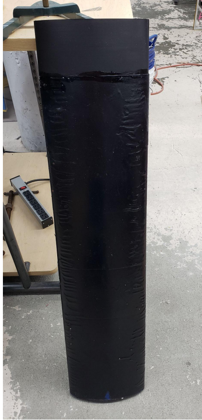
Figure 19: Wing assembly with paint and Flex Seal
