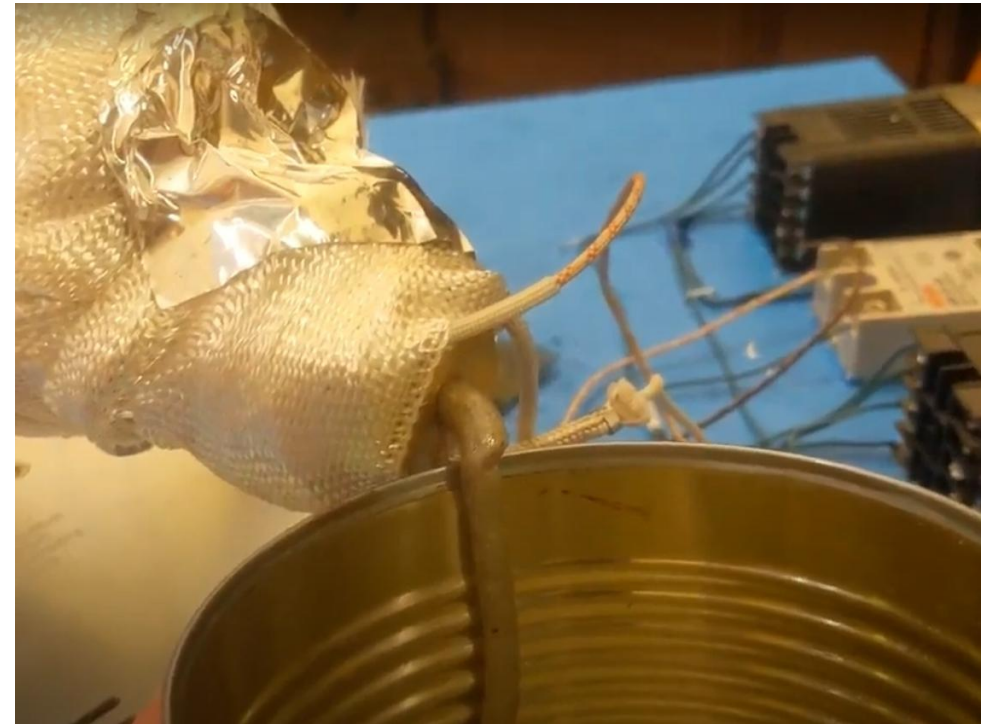
Extruding densified polystyrene
