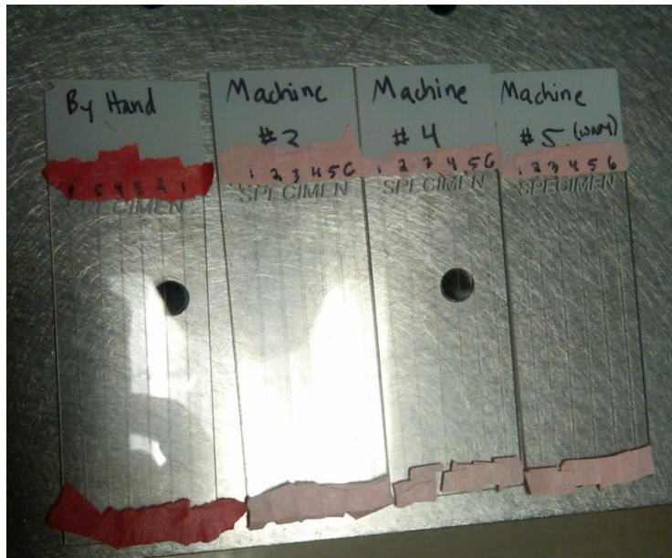
Figure 101: Slide setup for Microscopic Diameter Measurement
