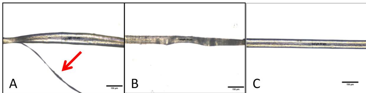
Figure 100: Microscope images showing (A) contaminants in the threads, (B) diameter bulging in wavy thread and (C) consistent diameter of straight thread
