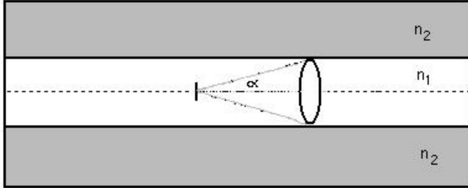
Figure 10: Solid Angle Trapped in Fiber
