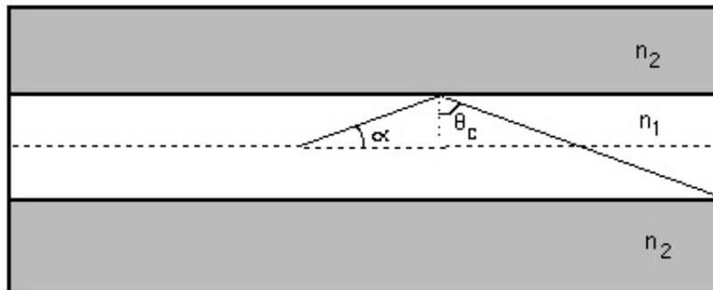
Figure 1: Total Internal Reflection in a fiber
