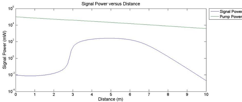
Figure 23: Signal and Pump Powers, 80 Bin ASE Model
