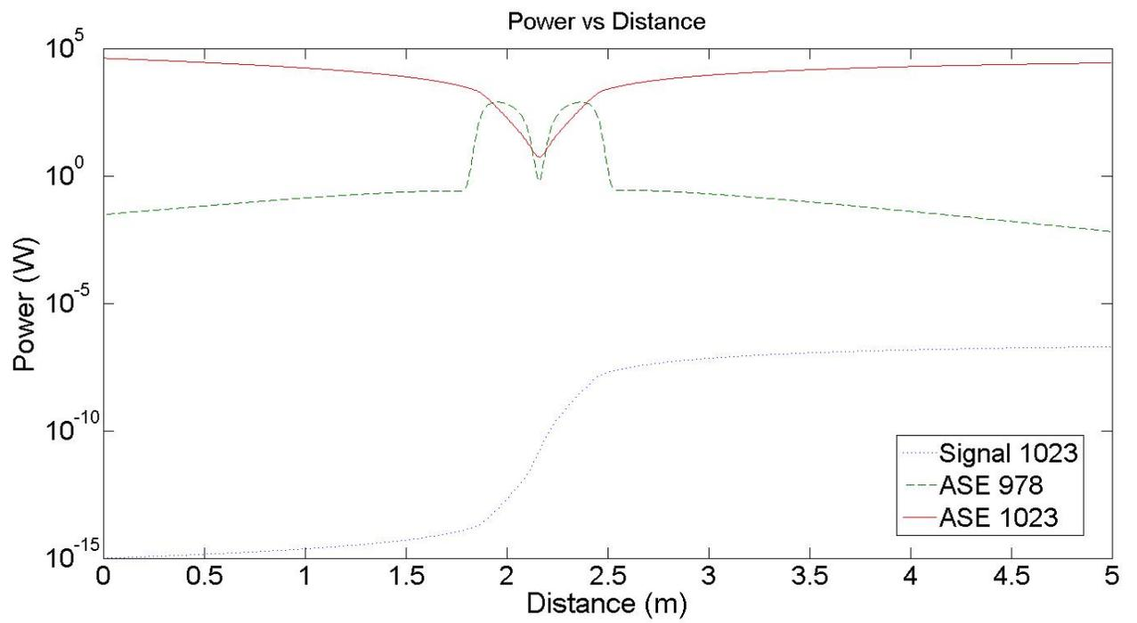
Figure 39: Signal, 978 and 1023 nm ASE Power vs Distance,  $P_s = 10^{-15}$  W,  $P_p = 10^5$  W
