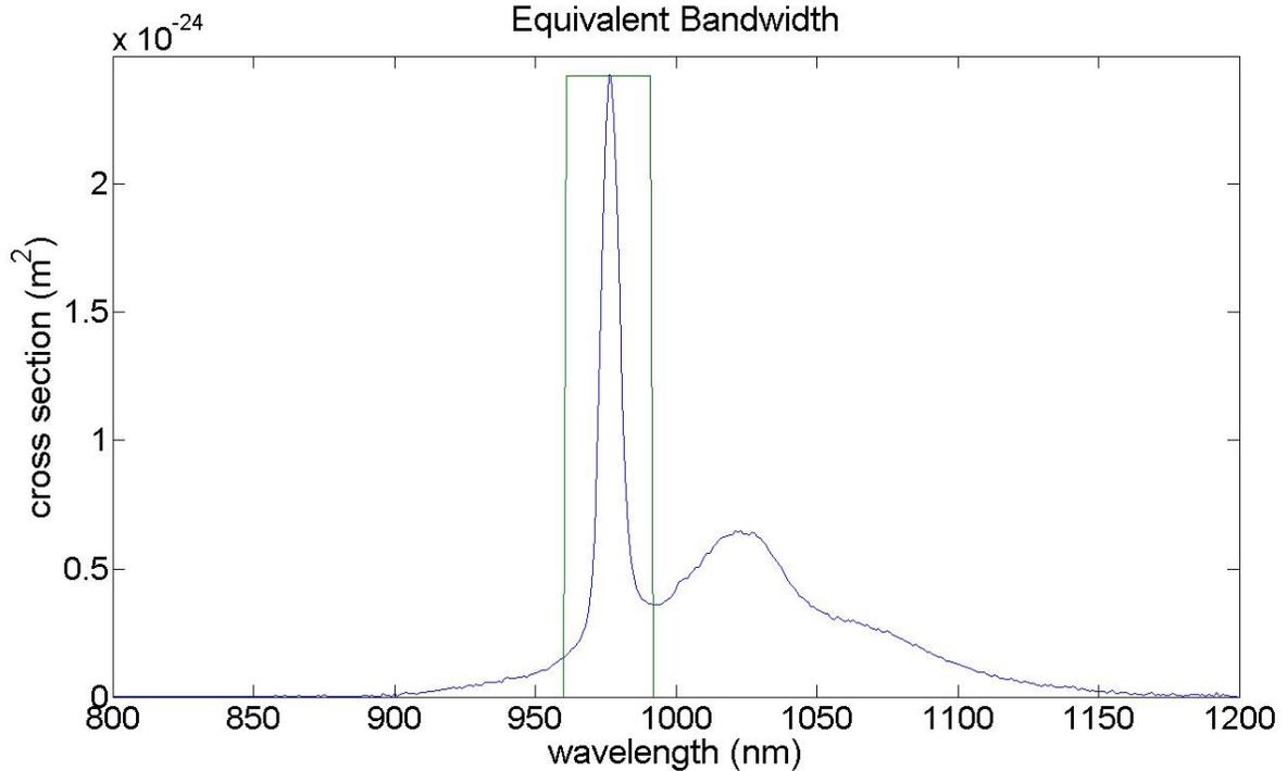
Figure 16: Emission Cross Section Spectrum with Equivalent ASE Band, One Bin
