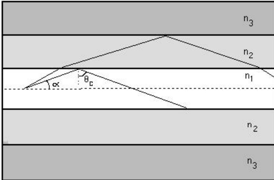
Figure 12: ASE trapped in cladding
