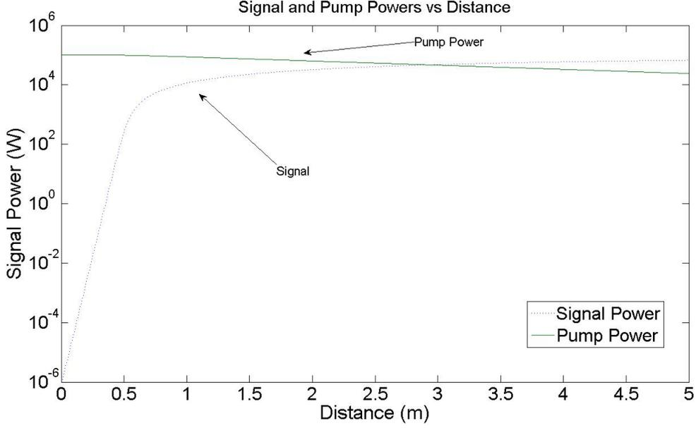
Figure 27: Pump and Signal Power vs. Distance,  $P_p = 10^5$  W and  $P_s = 10^{-6}$
