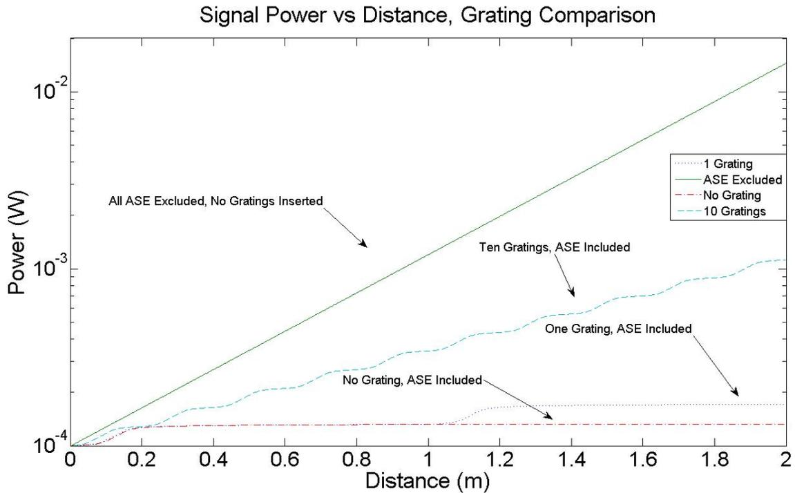
Figure 72: Signal Power vs Distance with Insertion of Diffraction Gratings,  $P_p = 10^3$  W and  $P_s = 10^{-4}$
