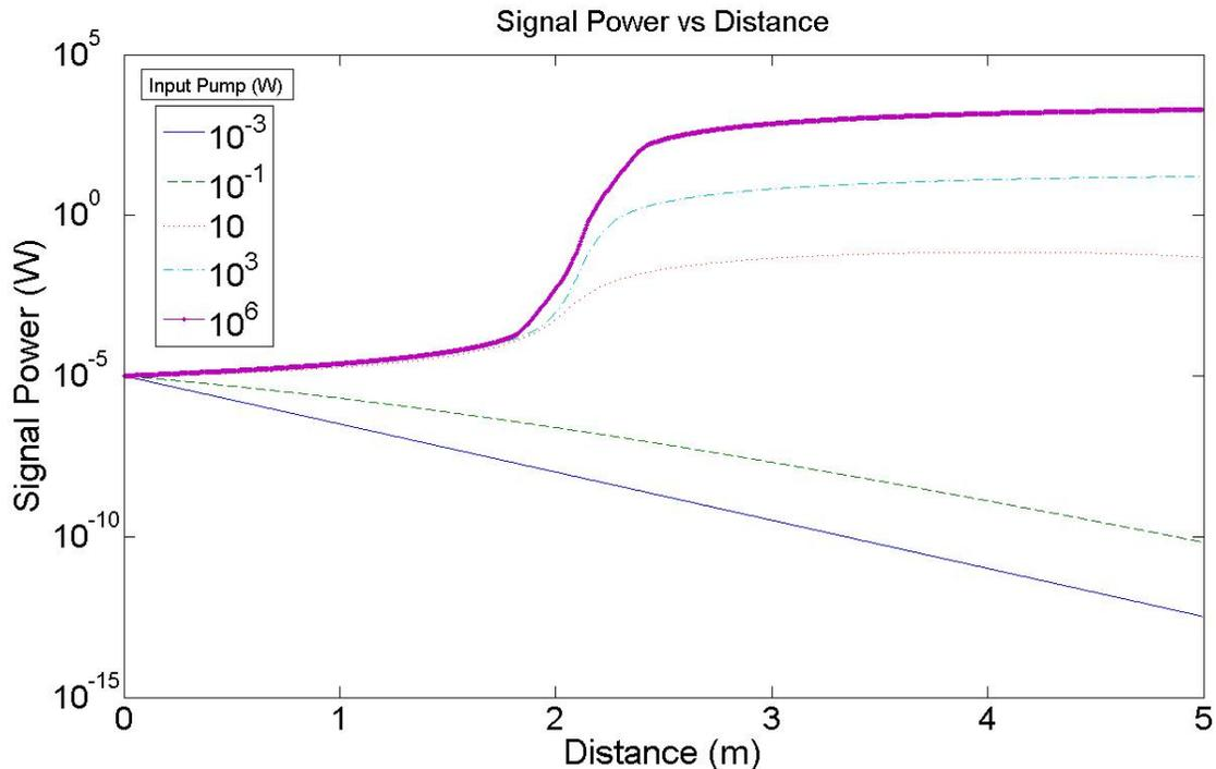
Figure 43: Signal Power vs Distance,  $P_s = 10^{-5}$  W, Varied Pump
