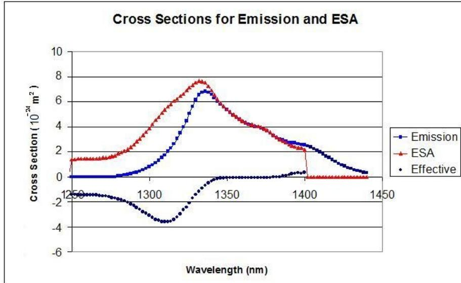
Figure 7: Effective Cross Section Due to ESA, Neodymium Doped in Silica Host Glass
