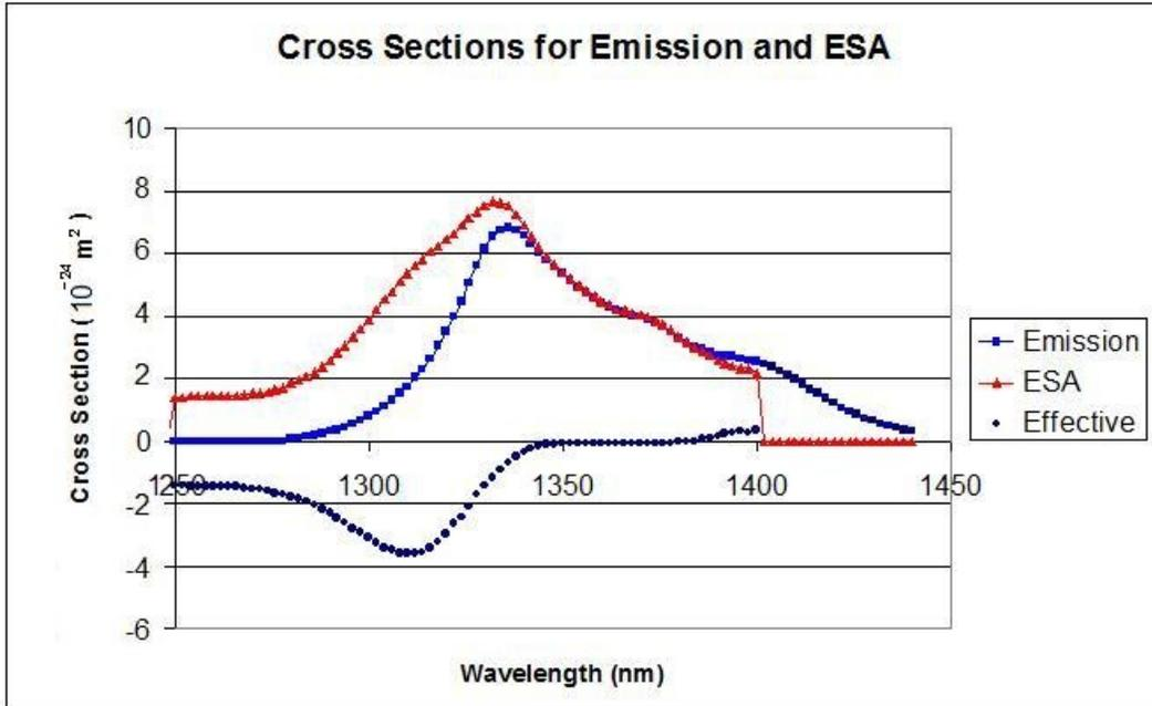
Figure 55: ESA and Effective Cross Section for Nd Near 1330 nm
