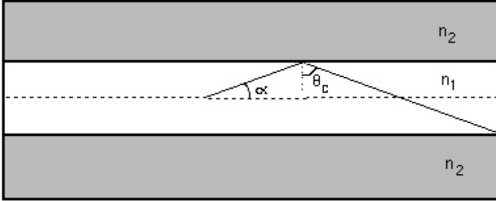
Figure 11: Relation of Critical Angle to Half Angle
