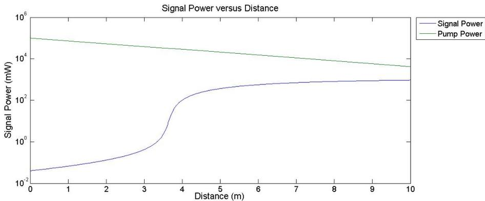
Figure 20: Signal and Pump Powers, Two Bin ASE Model
