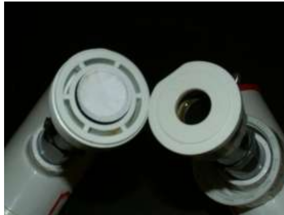
Figure 5: Threaded Flange with Membrane in Place
