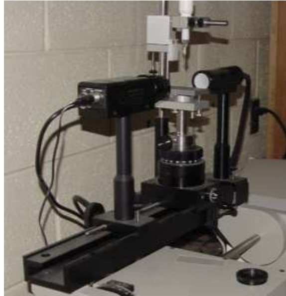
Figure 3: Sample Goniometer Equipment Setup
