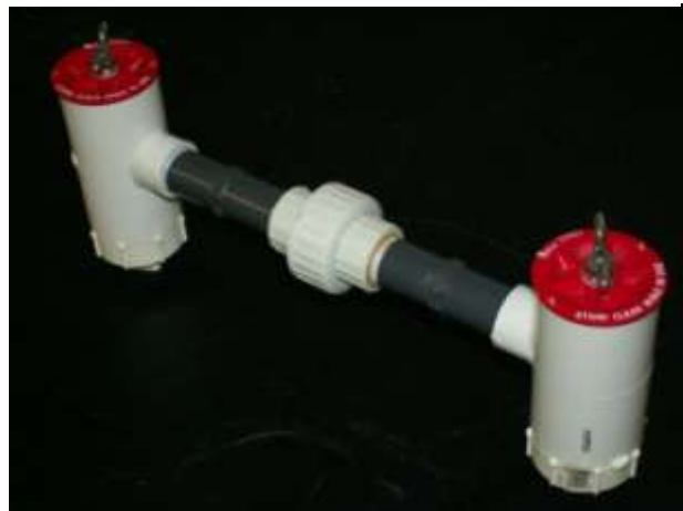
Figure 4: Test Apparatus with Two Reservoirs and a Coupling Flange
