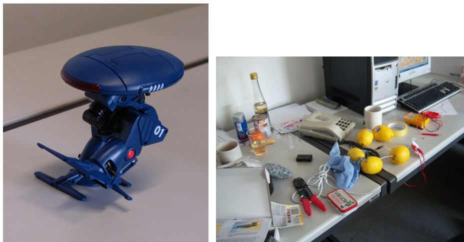
Figure 3 Lemon Battery Demonstration
