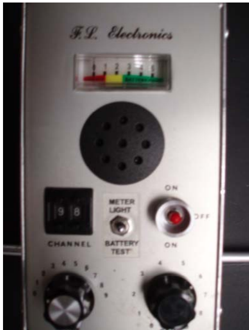
Figure 17: Close Up of Radio Control Box
