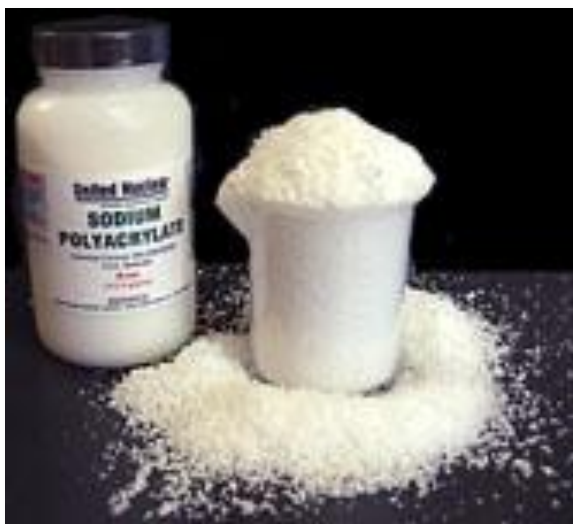
Figure 8-Sodium polyacrylate powder after absorbance
