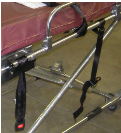
Figure 25- A closer look at the seatbelts and how they are not anchored along the bar
