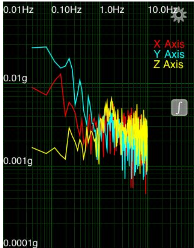
Figure 47-Frequency vs. Time graph of 2nd trial on smooth road with Akton Polymer
