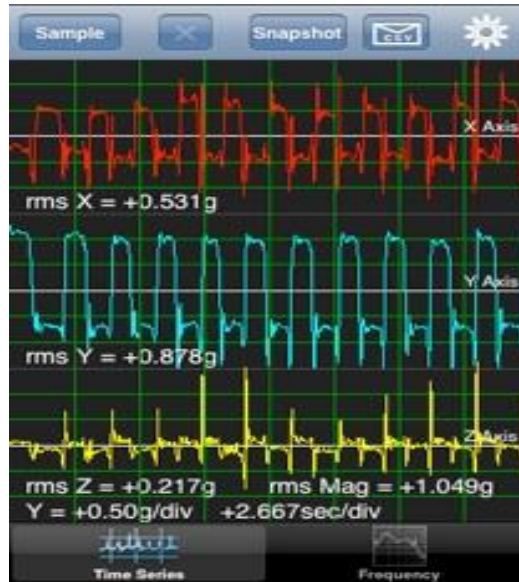
Figure 35-Snapshot of a trial run performed on time series menu of the iPhone Vibration App
