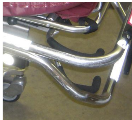
Figure 23- The levers at the foot of the stretcher
