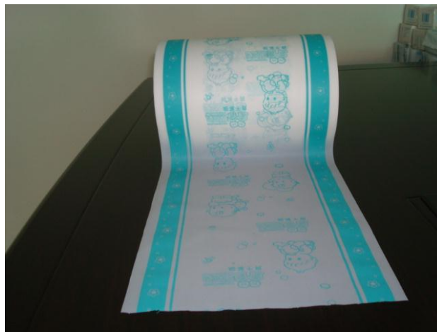
Figure 5-A thin layer of polyethylene back- sheeting
