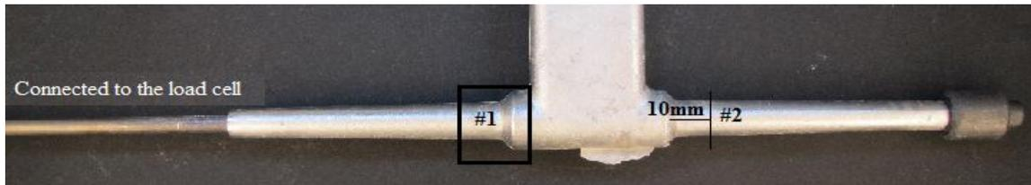
Figure 10: The positions of samples for microstructure analysis
