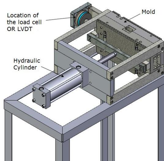
Figure 3: Mold assembly
