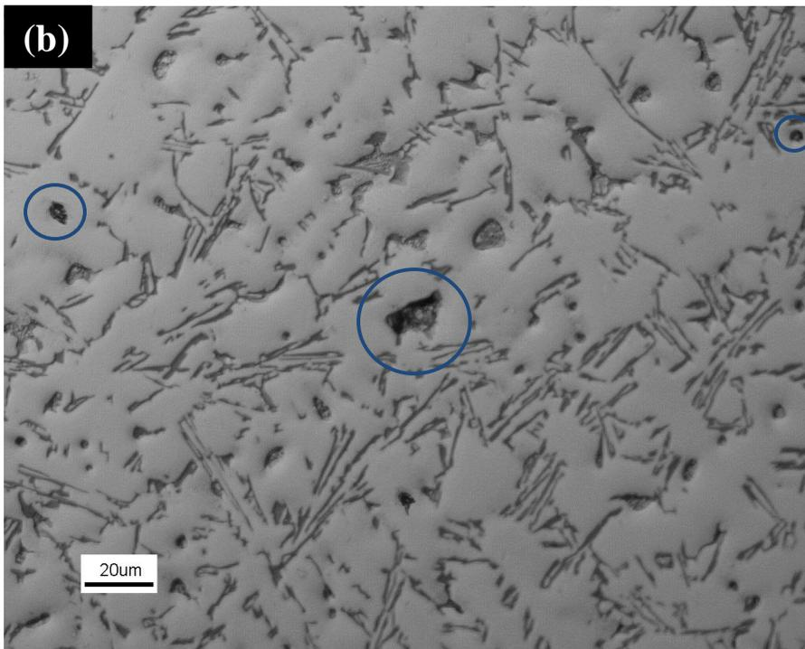
Figure 27: (a) Optical micrograph of pure A380.1; (b) Optical micrograph of A380.1 with added oxide inclusion. The circle points out the oxides.
