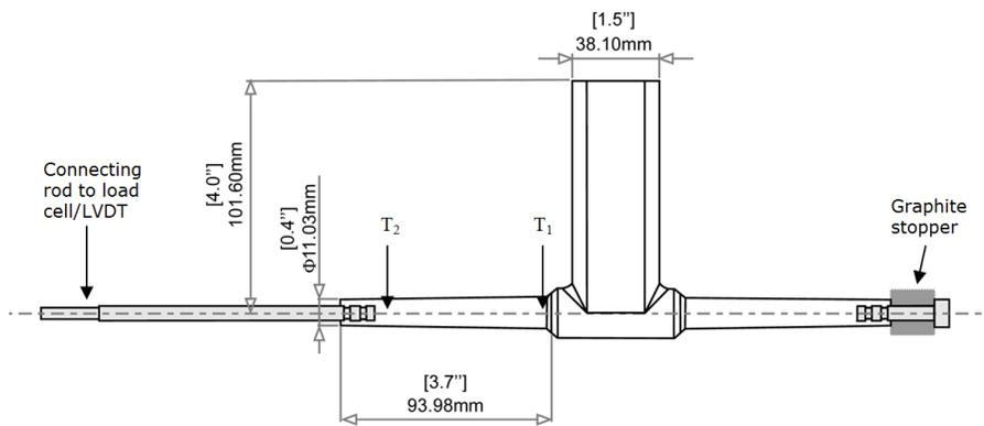
Figure 4: Casting dimensions
