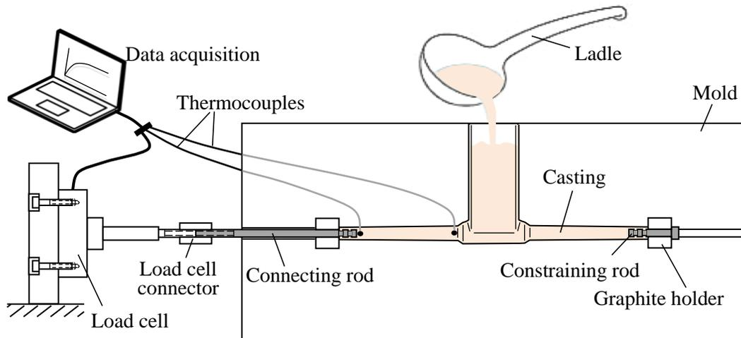
Figure 2: Diagram of experimental set-up
