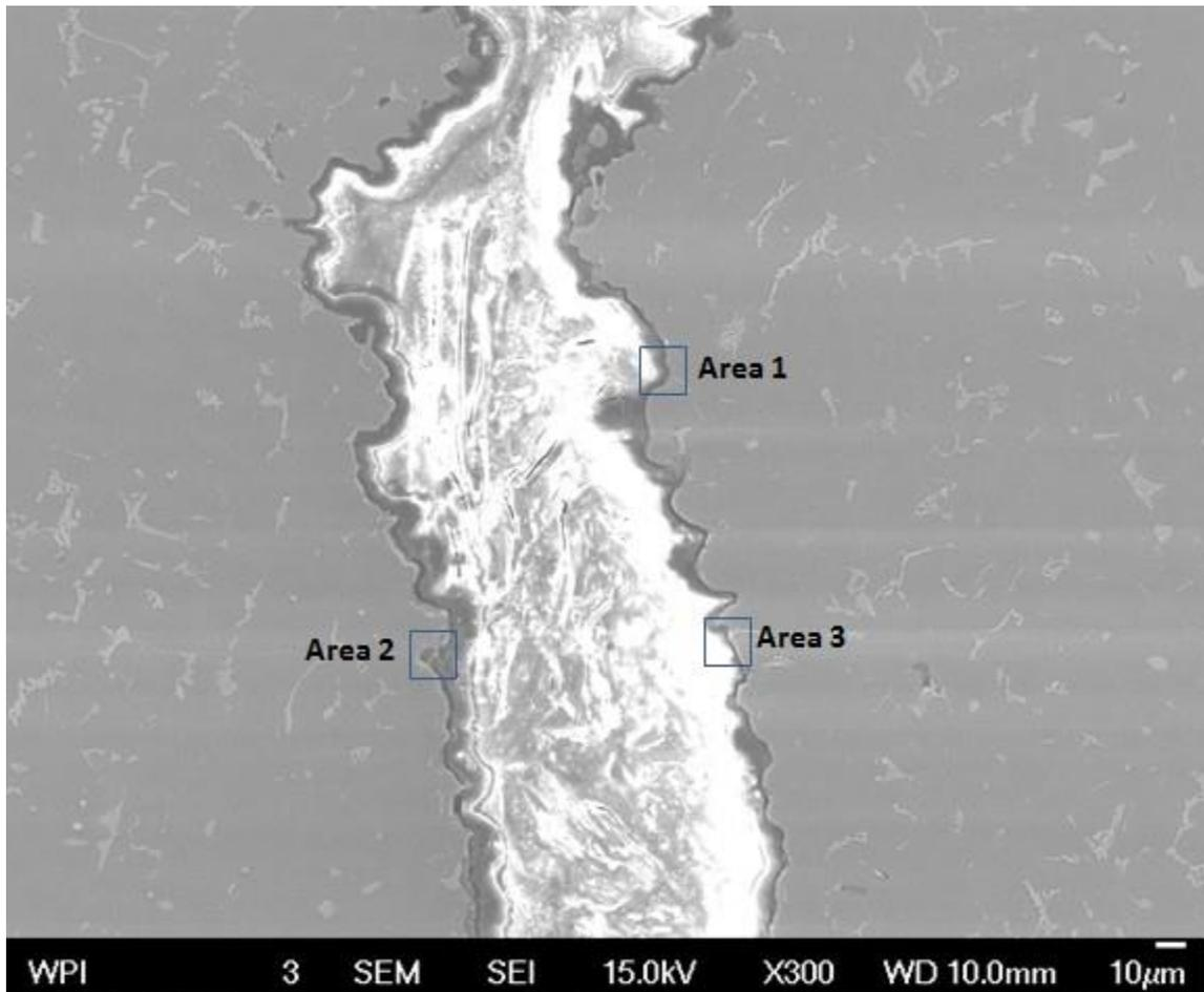
Figure 28: SEM image of the crack and areas analyzed in A380.1 with added oxides
