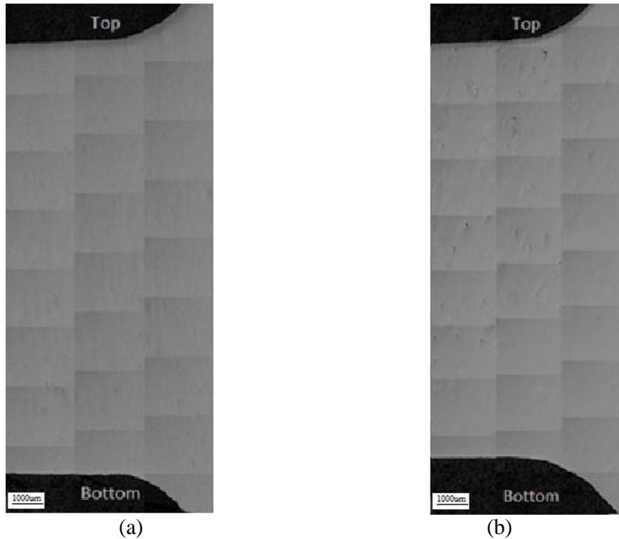
Figure 23: (a) Mosaic optical micrograph showing the longitudinal cross section of the neck region of pure A380.1; (b) Mosaic micrograph in the neck region of A380.1 modified with Sr
