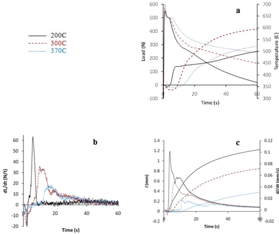
Figure 8: (a) Temperature and load development as a function of time for M206 at different mold temperatures, temperature measured at centerline of the rod at the riser end (Tc1); (b) Derivative of load vs. time curves; (c) Measured displacement and its derivative as a function of time
