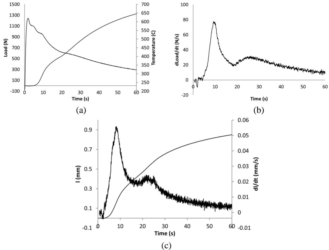
Figure 22: (a) Load development and temperature vs. time for A380.1 modified with strontium; (b) Derivative of load vs. time; (c) Displacement and its derivative vs. time
