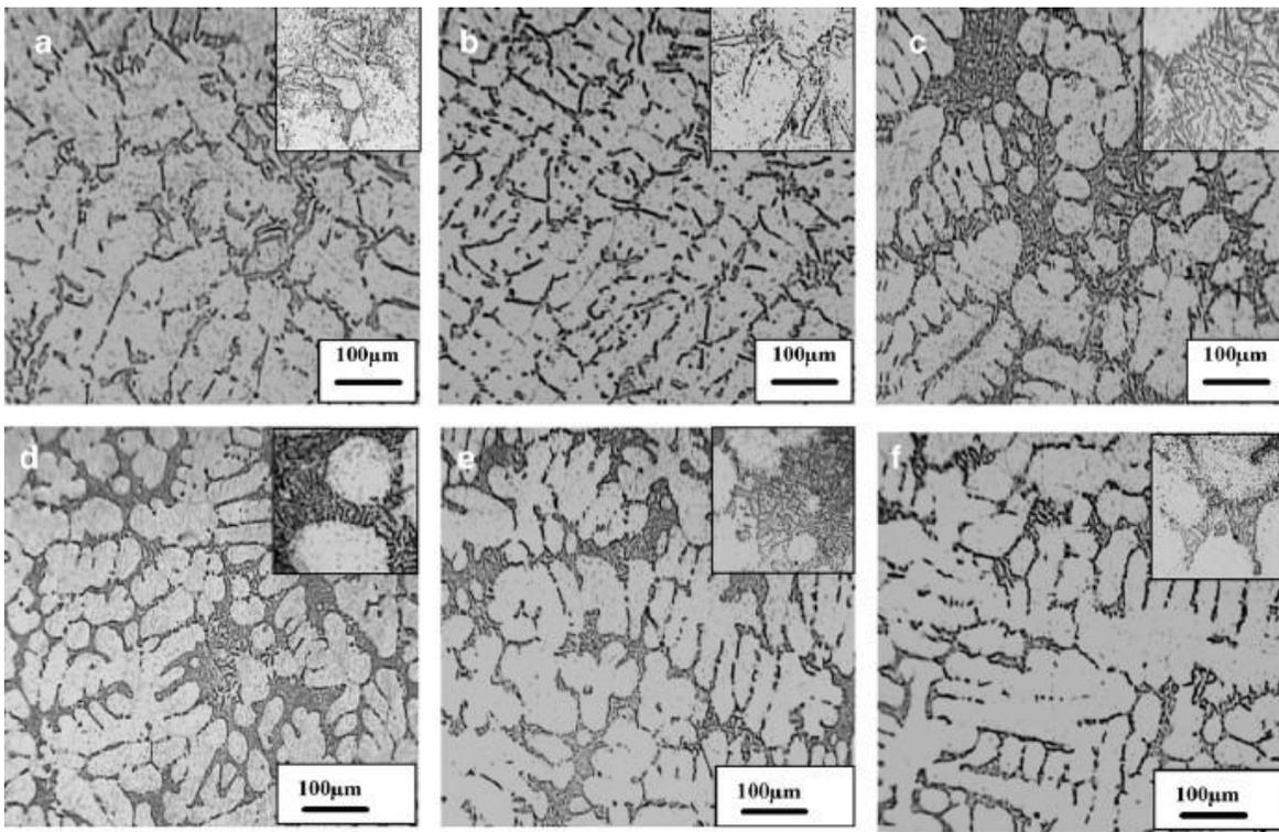
Figure 1: Optical micrograph of A357: (a) non-modified, (b) modified with 0.01%Sr, (c) modified with 0.02%Sr, (d) Modified with 0.03%Sr, (e) modified with 0.05%Sr, and (f) modified with 0.1%Sr<sup>[16]</sup>
