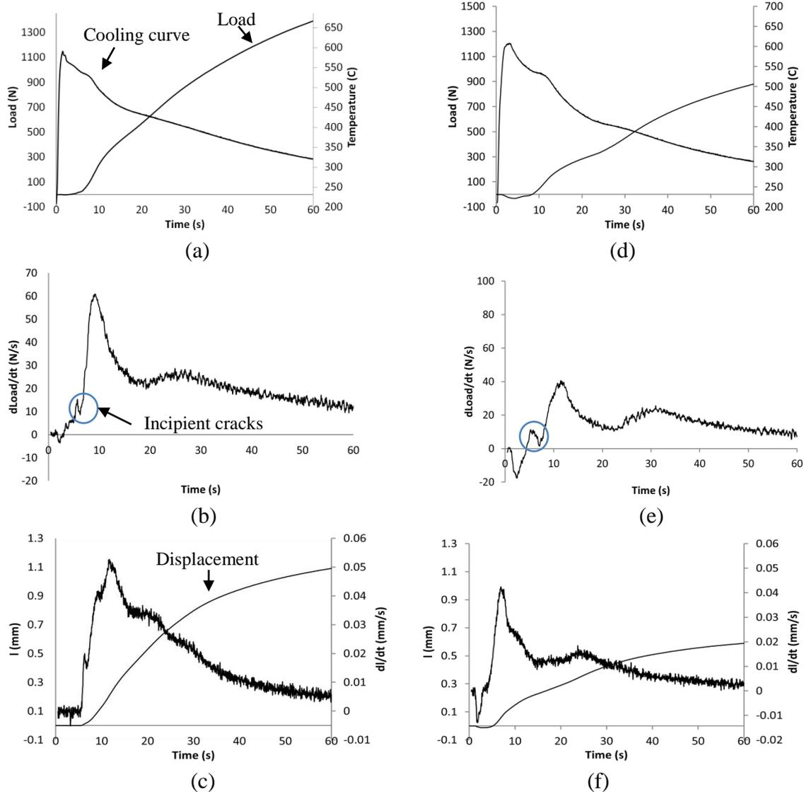
Figure 12: (a) Load development and temperatures vs. time for A380.1; (b) Derivative of load vs. time curve for A380.1; (c) Displacement and its derivative vs. time for A380.1. (d) Load development and temperatures vs. time for A390; (e) Derivative of load vs. time curve for A390; (f) Displacement and its derivative vs. time for A390
