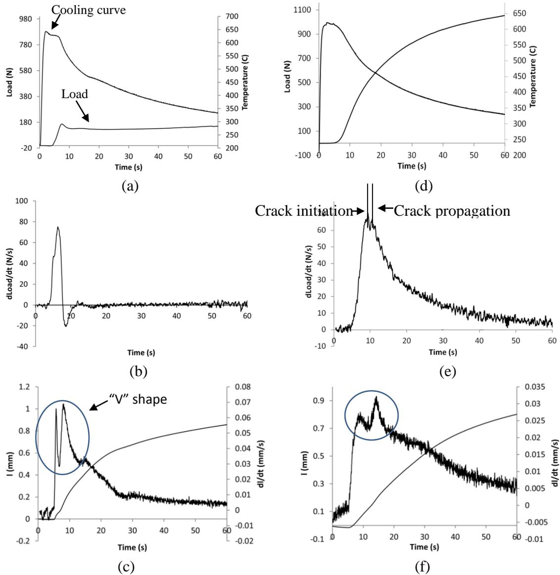
Figure 16: (a) Load development and temperatures vs. time for 6061; (b) Derivative of load vs. time curve for 6061; (c) Displacement and its derivative vs. time for 6061; (d) Load development and temperatures vs. time for 7075; (e) Derivative of load vs. time curve for 7075; (f) Displacement and its derivative vs. time for 7075
