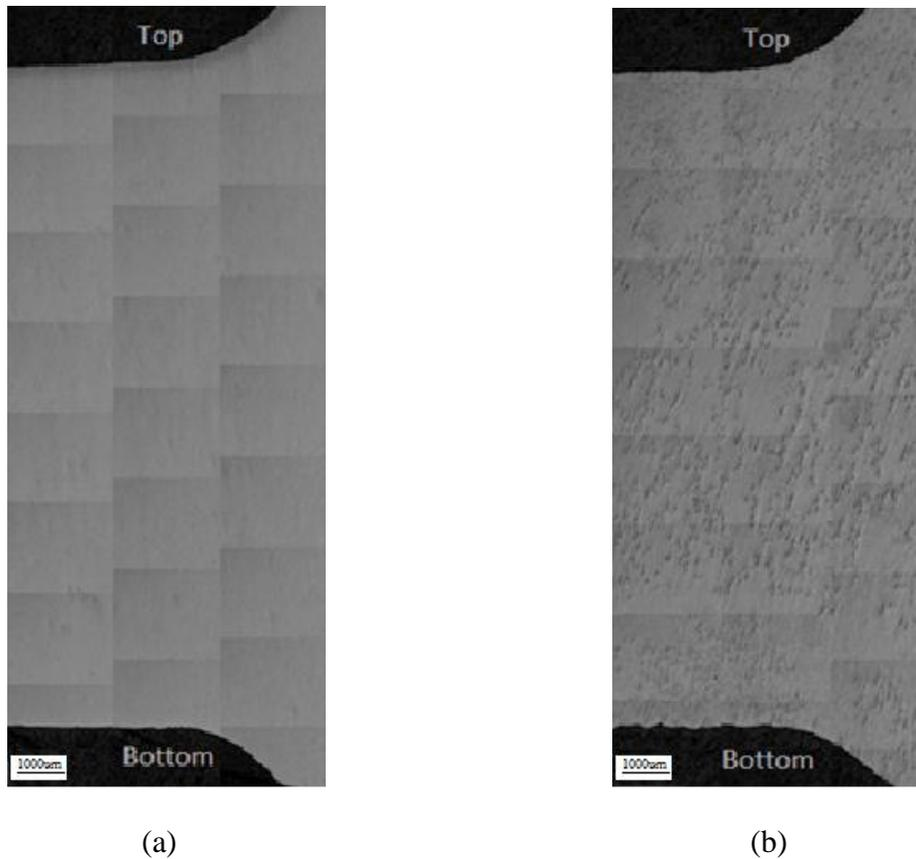
Figure 13: (a) Mosaic optical micrograph showing the longitudinal cross section of the neck region of A380.1; (b) Mosaic micrograph in the neck region of alloy A390
