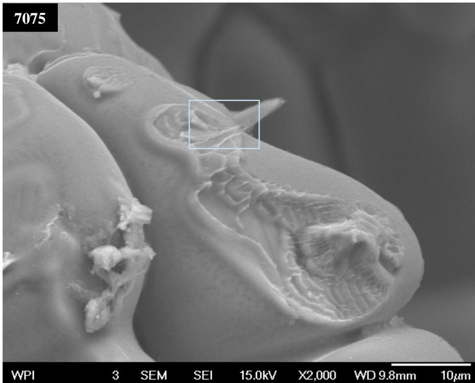
Figure 21: The fracture SEM image of 6061 and 7075 at high magnification
