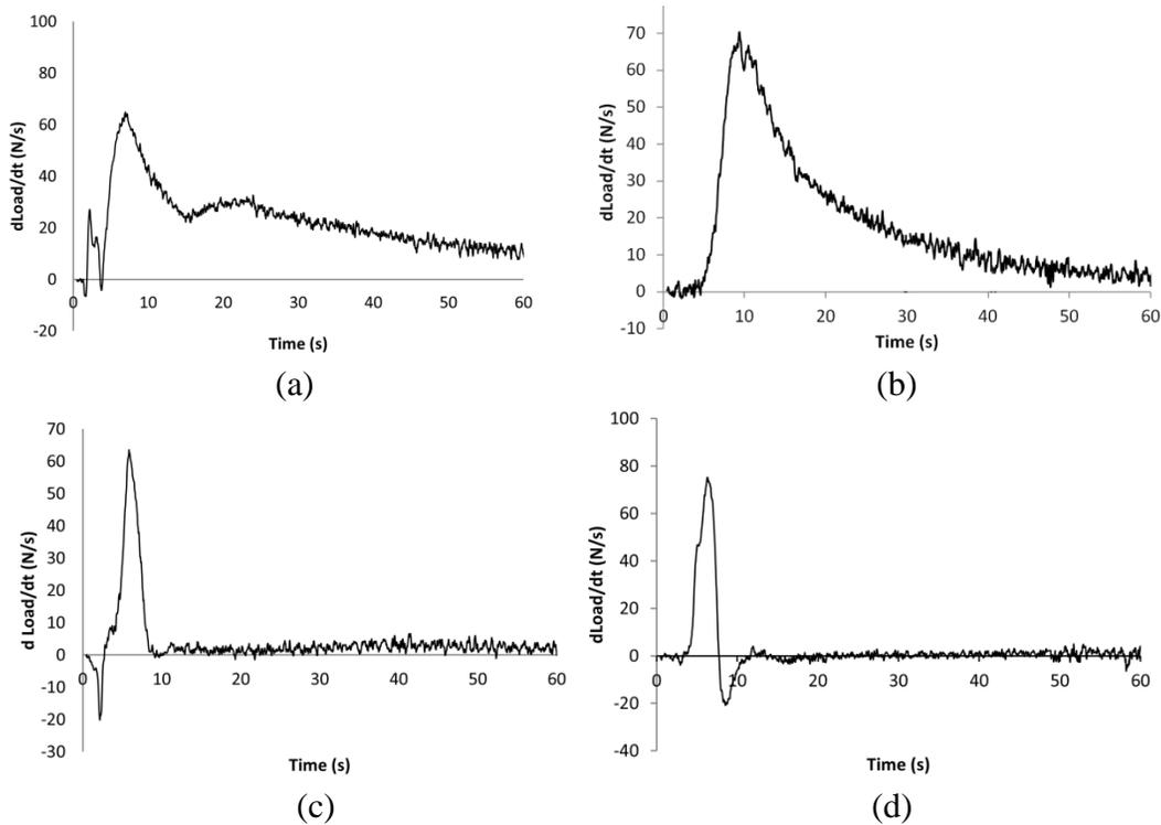
Figure 34: Derivative of load vs. time: (a)A380.+oxides, (b)7075, (c)M206 <sup>[24]</sup>, (d)6061.
