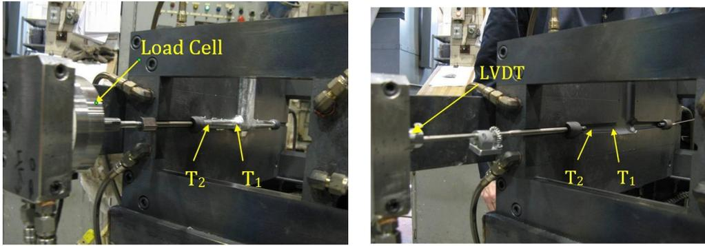
Figure 5: Load cell and LVDT setup
