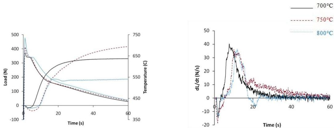
Figure 9: Left diagram: Temperature and load development as a function of time for M206 at different pouring temperatures, temperature measured at centerline of the rod at the riser end; Right diagram: Derivative of load vs. time curves
