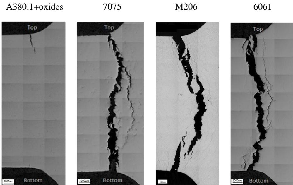
Figure 33: Crack images for A380.1+oxides, 7075, M206<sup>[6]</sup>, and 6061.
