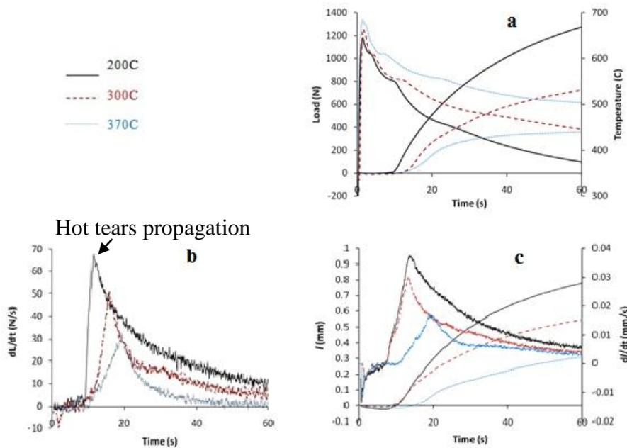
Figure 7: (a) Temperature and load development as a function of time for A356 at different mold temperatures, temperature measured at centerline of the rod at the riser end (Tc1); (b) Derivative of load vs. time curves; (c) Measured displacement and its derivative as a function of time
