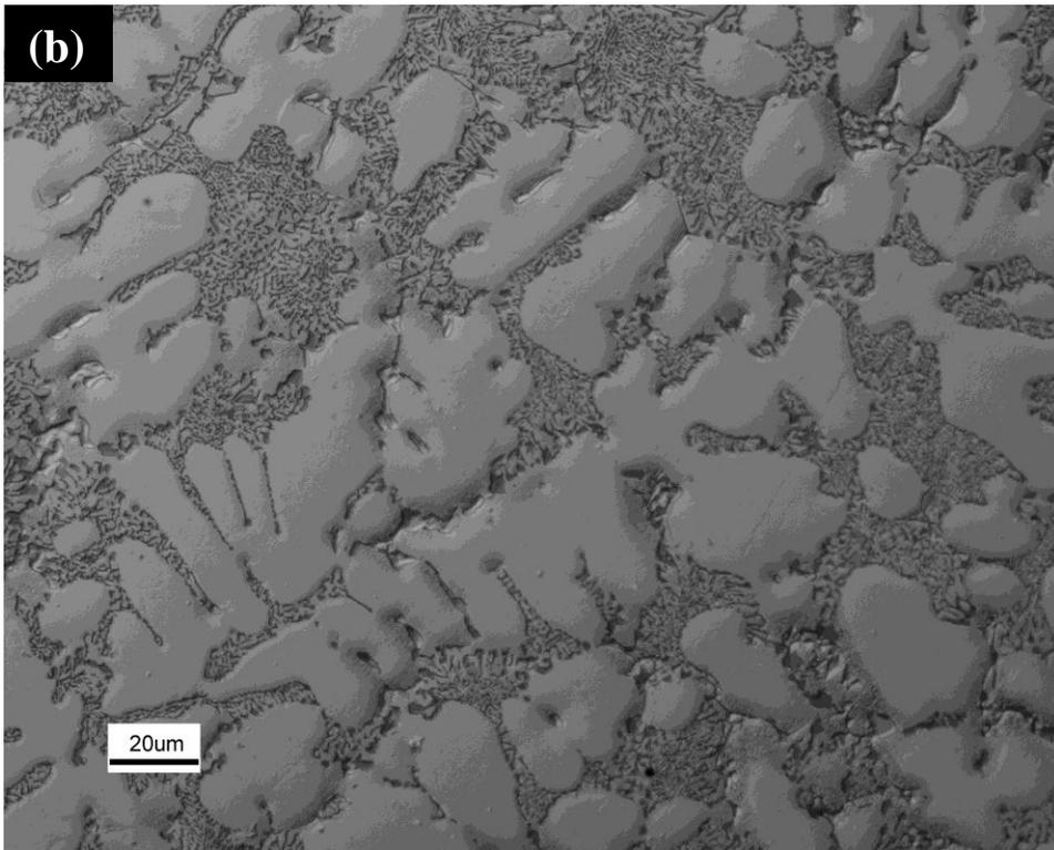
Figure 24: (a) Optical micrograph of pure A380.1; (b) Optical micrograph of A380.1 modified with Sr
