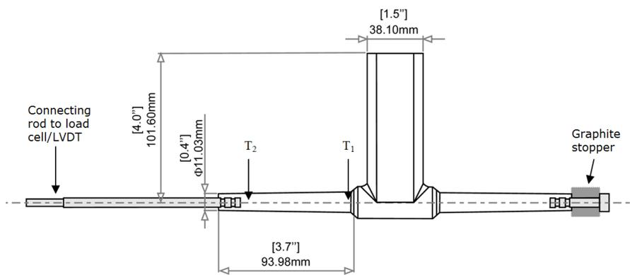
Figure 4: Casting dimensions
