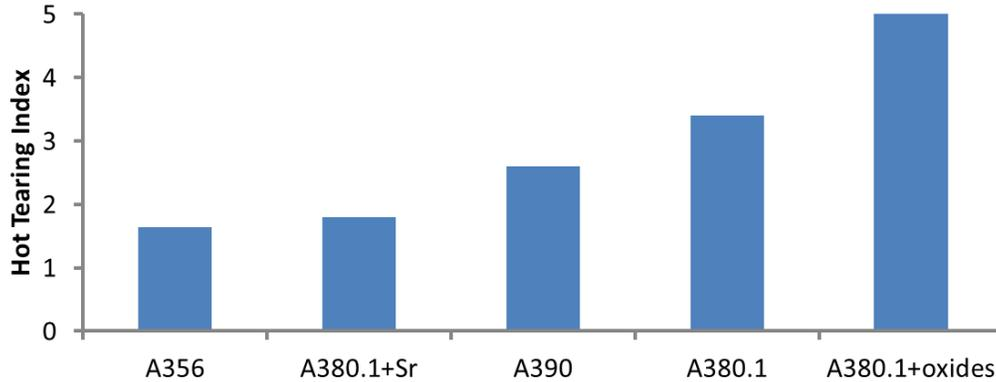
Figure 32: Hot tearing index for different alloys in the no-crack part
