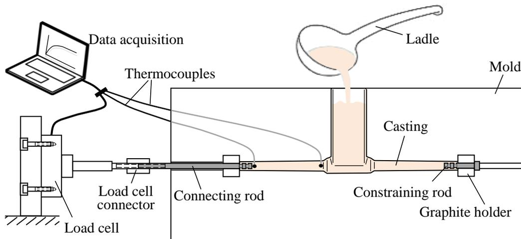
Figure 2: Diagram of experimental set-up
