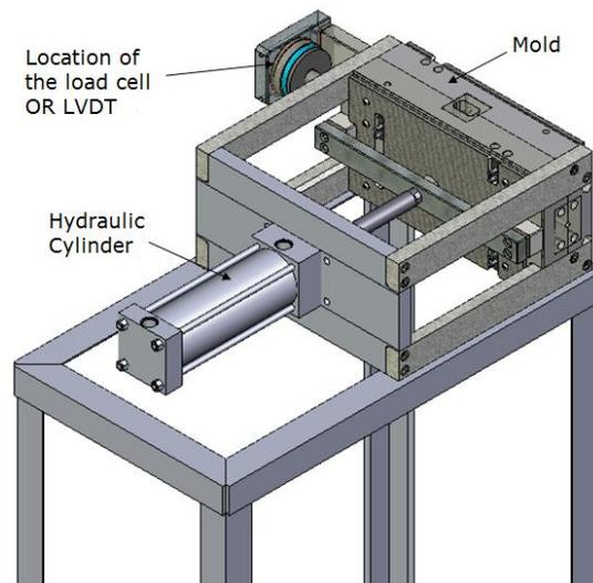
Figure 3: Mold assembly
