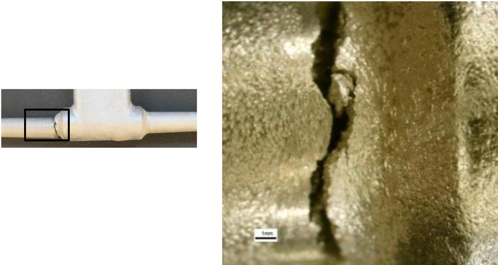
Figure 17: (a) Photographs of the constrained casting showing cracking locations of 6061;
