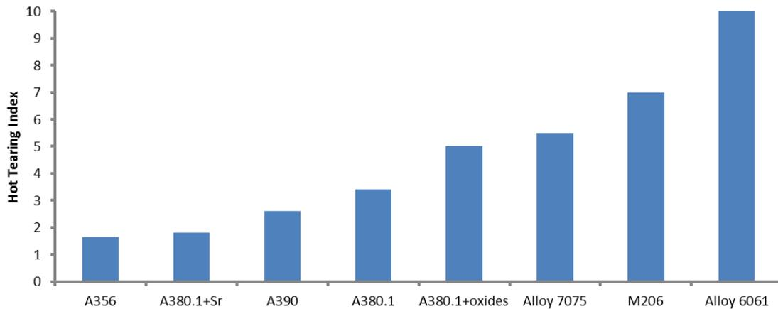
Figure 36: Hot tearing index for different alloys
