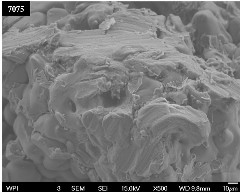
Figure 20: The brittle fracture SEM images of 6061 and 7075 at low magnification
