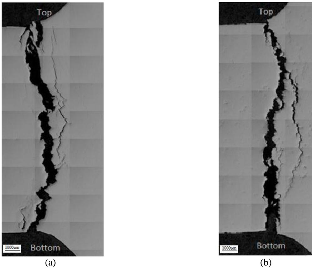
Figure 18: (a) Mosaic optical micrograph showing the longitudinal cross section of the neck region of 6061; (b) Mosaic micrograph showing hot tears in the neck region of 7075
