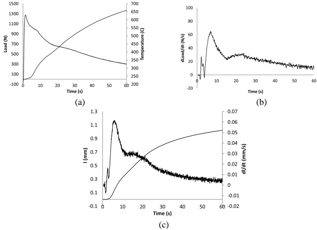
Figure 25: (a) Load development and temperature vs. time for A380.1 with added oxides; (b) Derivative of load vs. time; (c) Displacement and its derivative vs. time.
