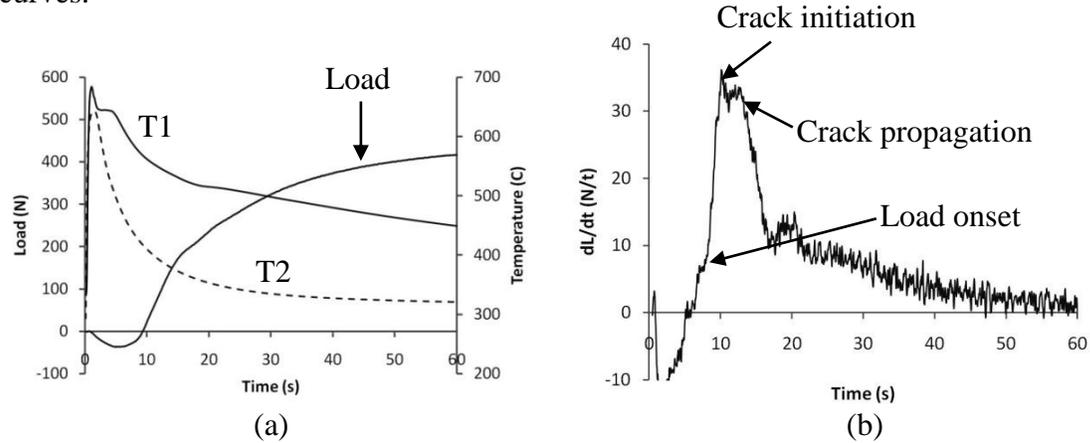
Figure 11: (a) Temperatures and load development as a function of time for M206; (b) Derivative of load vs. time curves
