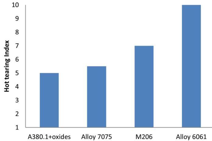
Figure 35: Hot tearing index for different alloys in the large-crack part
