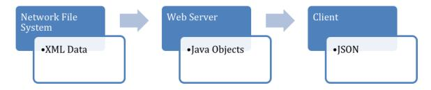
**Figure 8: Data Format Conversion Flowchart**
