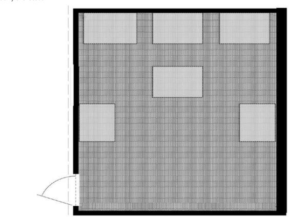
The fire patterns that were classified as being generated by a PLUME or as UNDETERMINED will be considered as the area of origin. IF there is only one of these patterns, then this is the area of origin. IF there are two or more of these patterns, then your area of origin will need to encompass all of these plume and/or undetermined generated patterns. Please select (click) on the region(s) of the diagram that encompass the area of origin for this fire.
