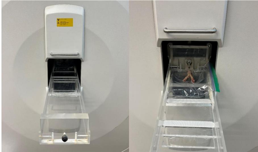
*Figure 7: (left) The SCANCO Medical XtremeCT with tray loaded on machine and pushed in all the way. (right) Example of how a sample can be loaded with a plastic zipper bag to create a gap between the tray and the sample.*
