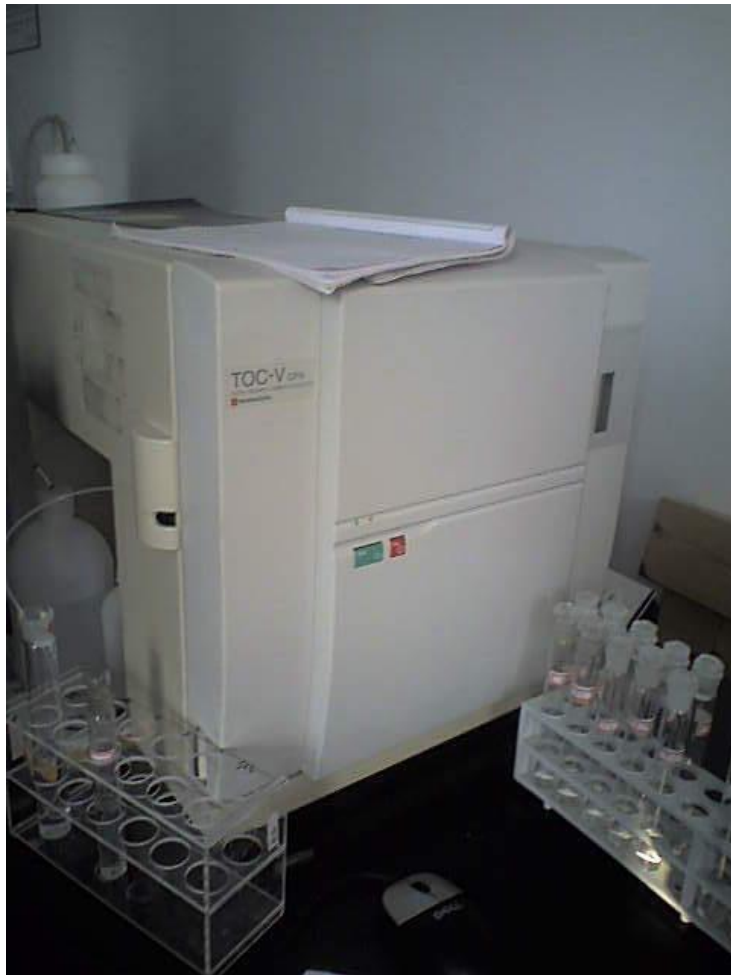
Figure 1 TOC-Vcpn machine used to measure total organic carbon
