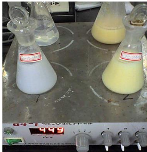
Figure 4. Solution after having been stirred for 24 hours and ready to be heated to 130°C 1) left front flask is the formation of control SBA-15 2) right front flask is the formation of SBA-15 loaded with iron nitrate
