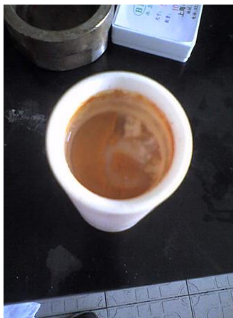
Figure 5. Formation of SBA-15 loaded with ferric nitrate after being heated at 130 degrees C to separate polymers from the mesoporous material
