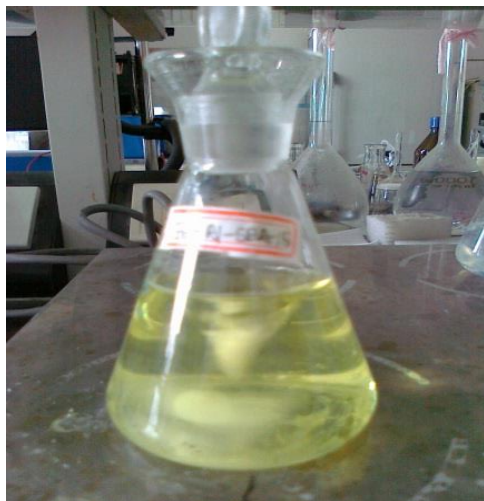
Figure 3. Dissolving of iron and TEOS in a solution containing the surfactant P-123
