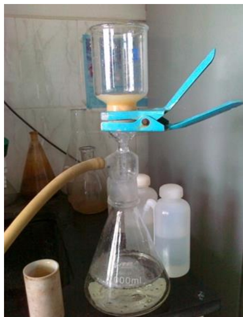
Figure 6. Vacuum filtration of SBA-15 loaded with ferric nitrate with distilled water to help remove polymers from particles
