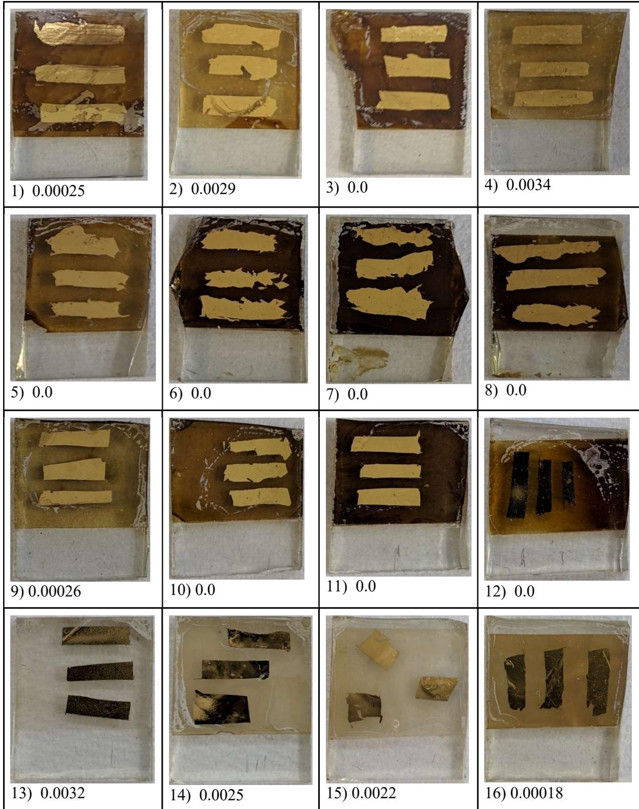
Figure 4: Sample Photos and Calculated % Efficiencies
