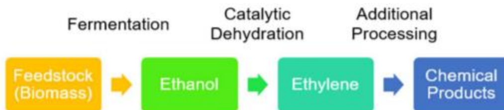
Figure 3: Process flow diagram of green ethylene production
