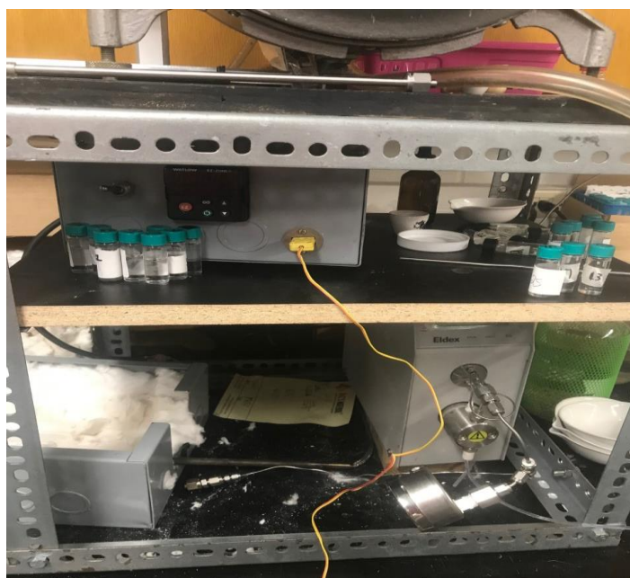
Figure 5: Ethanol feed, pump, heater, and reactor insulation (from right to left)
