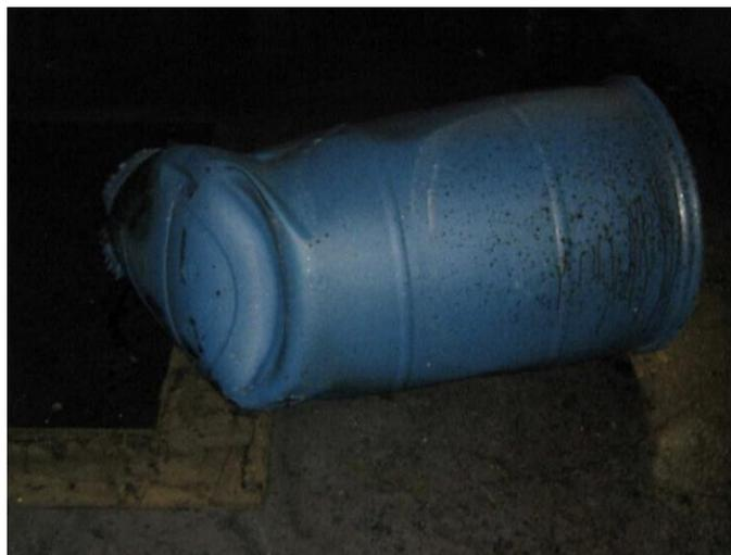
**Figure 2.** Over pressurized and overheated drum aftermath
