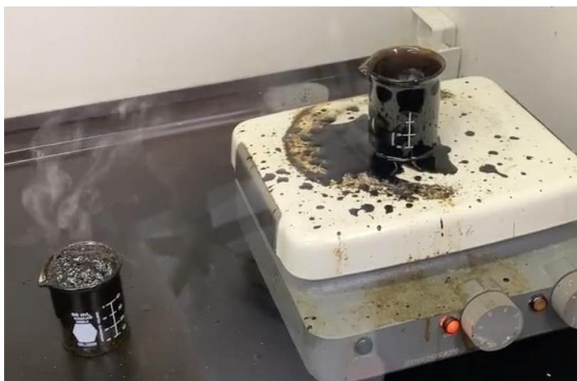
**Figure 14.** Mixed and unsealed reaction comparison test, PFA spill-over in mixed beaker (right).
