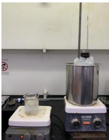
**Figure 17.** IC apparatus setup for determining heat capacity.
