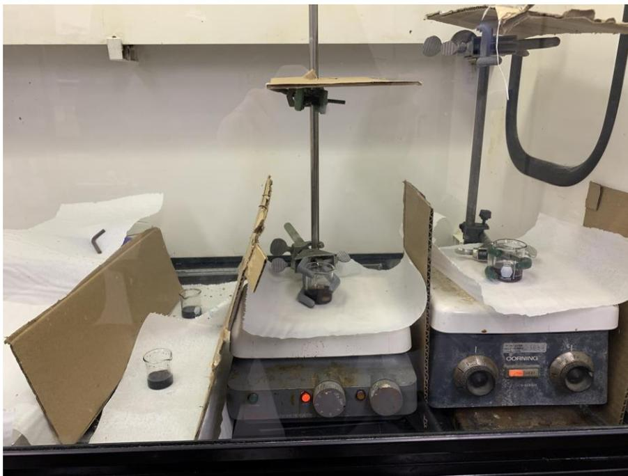
**Figure 20.** Experimental set up for changing the stir rate.
