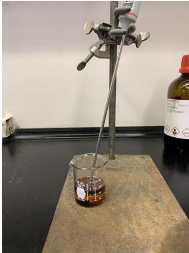
**Figure 9.** Initial open beaker experimental setup, 50mL beaker, 22mL of FA, 0.7mL of MSA.
