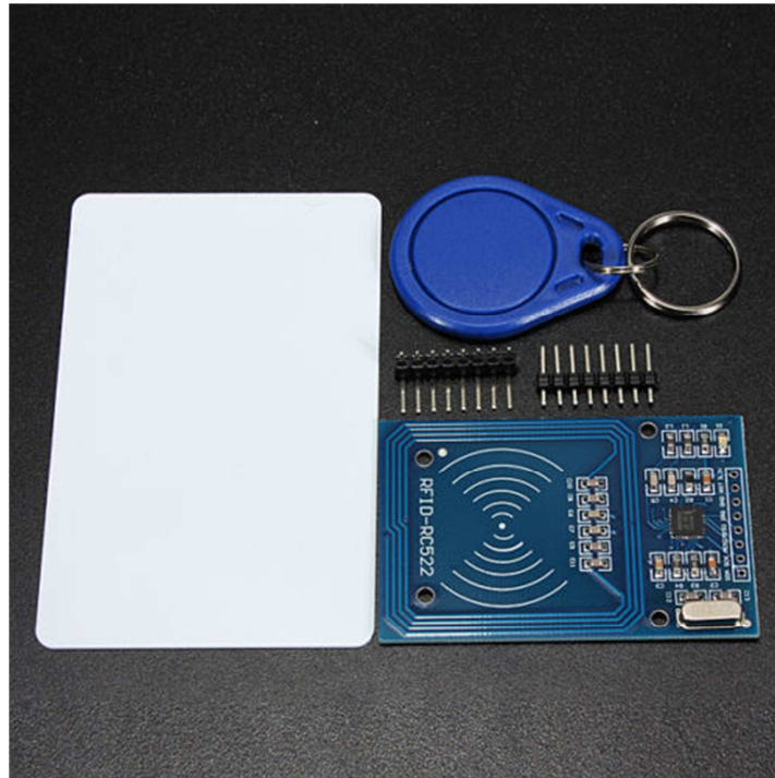
Figure 25: Mifare RFID RC522 Reader IC and Antenna module [41]
