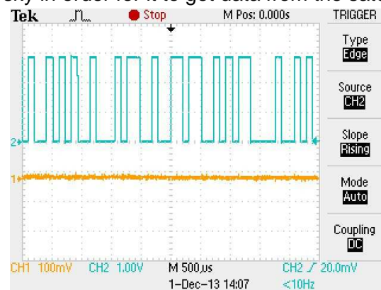
Figure 51: Scope photo of the GPS output
