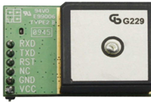
Figure 26: Skylab SKM53 GPS module [42]
