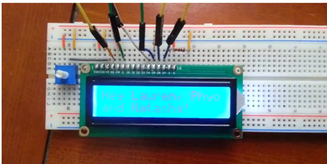
Figure 54: Working LCD display reads "Hey Lauren, Phyo and Natasha!"
