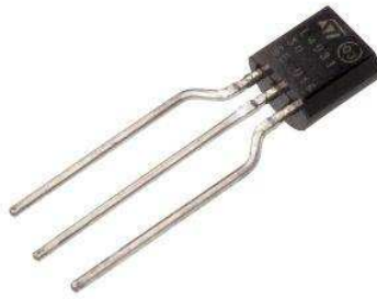
Figure 24: L4931 voltage regulator [40]
