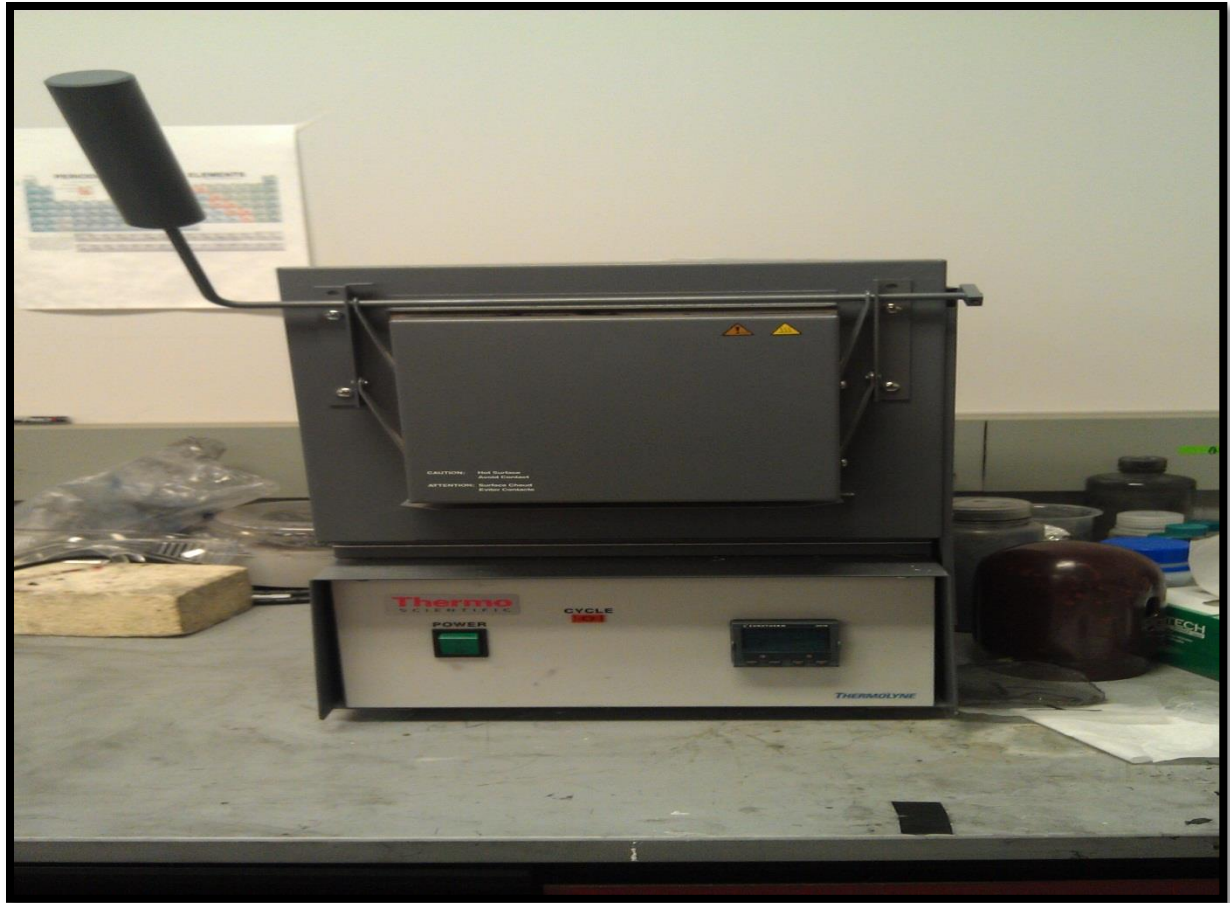
Figure 9 Furnace used for sintering LCO disks
