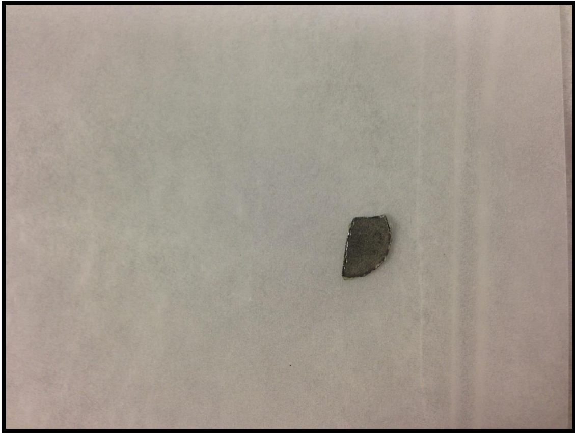
Figure 19 Cathode disk after LLTO sol evaporation
