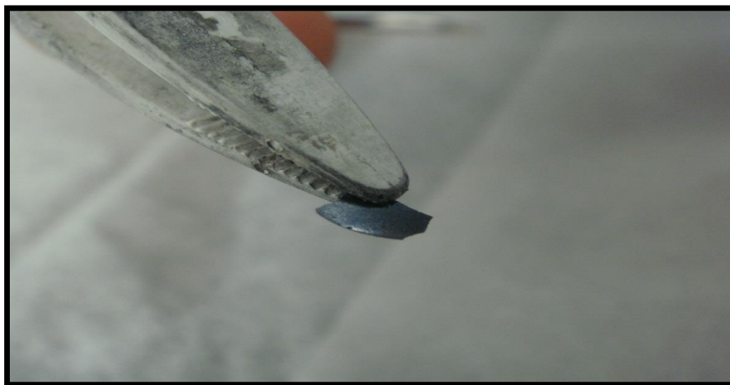
Figure 15 LCO cathode disk covered with LLTO Sol
