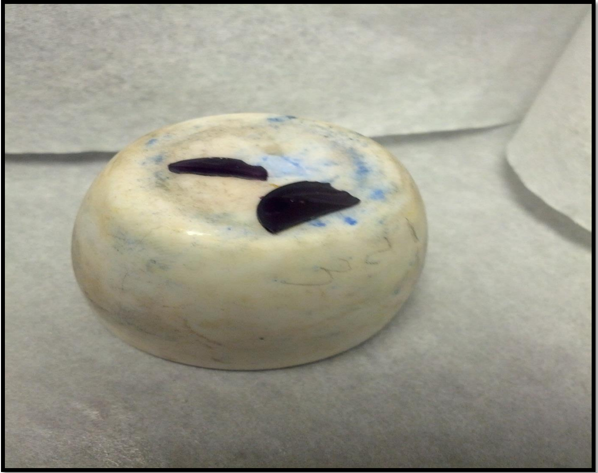
Figure 18 Evaporative LCO sol deposition (right), spin-coating deposition (left)
