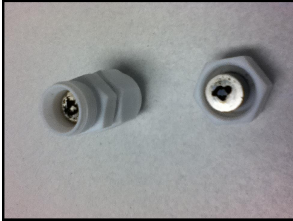
Figure 35 Disassembled battery after electrochemical testing
