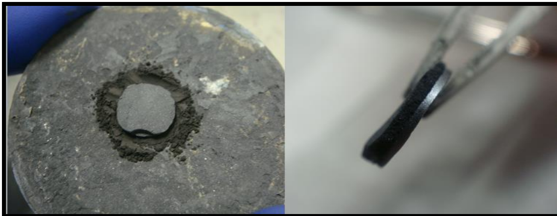
Figure 8 LCO Cathode disk before (left) and after (right) Sintering
