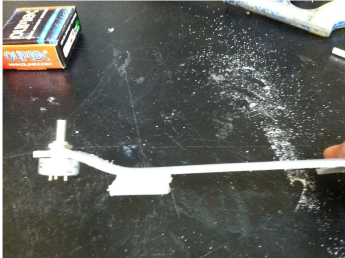
Figure 21 Side view of the upper leg support with potentiometer
