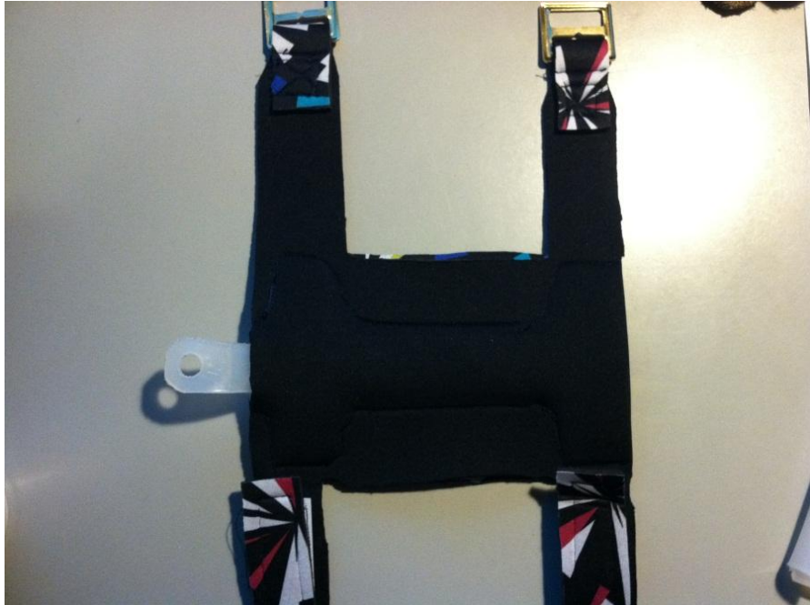
Figure 27. Upper leg portion with neoprene and adjustable Velcro straps
