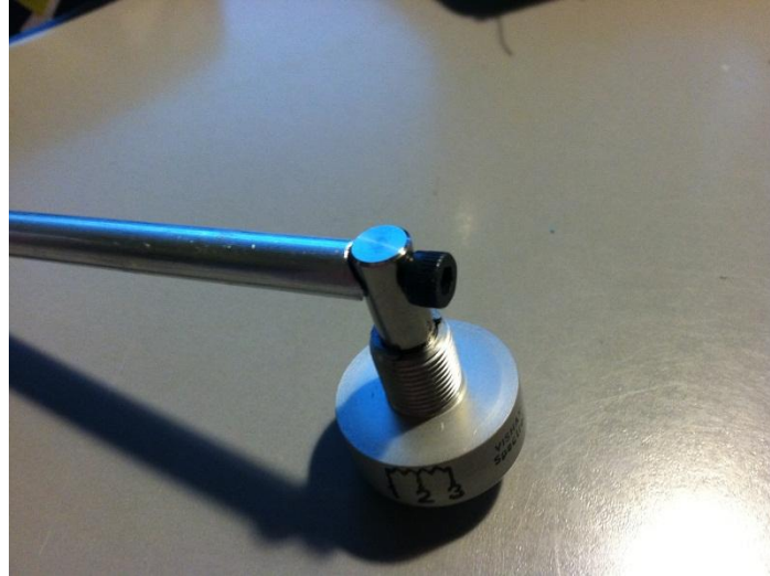
Figure 26. Potentiometer attached to the aluminum bar stock
