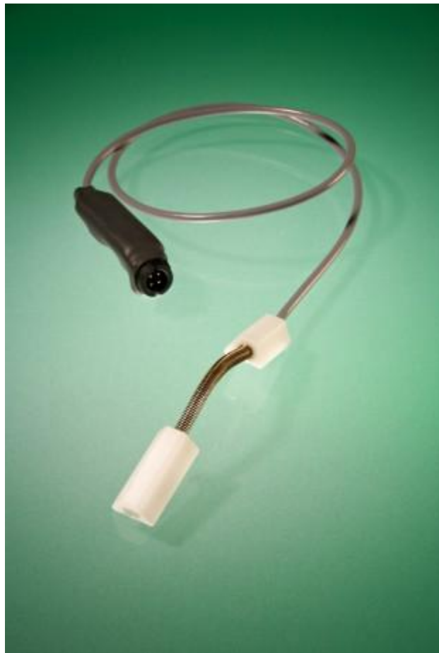
Figure 9. Biometrics Ltd. F35 Single-Axis Goniometer (Biometrics Ltd., 2011)
