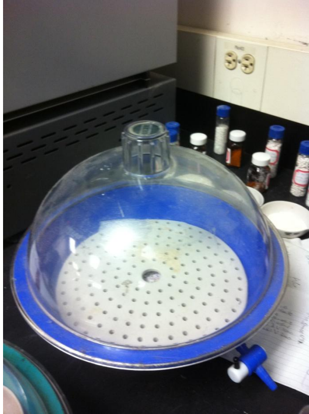
Figure 43: Cooler Plastic (Total Suspended Solids Test)
