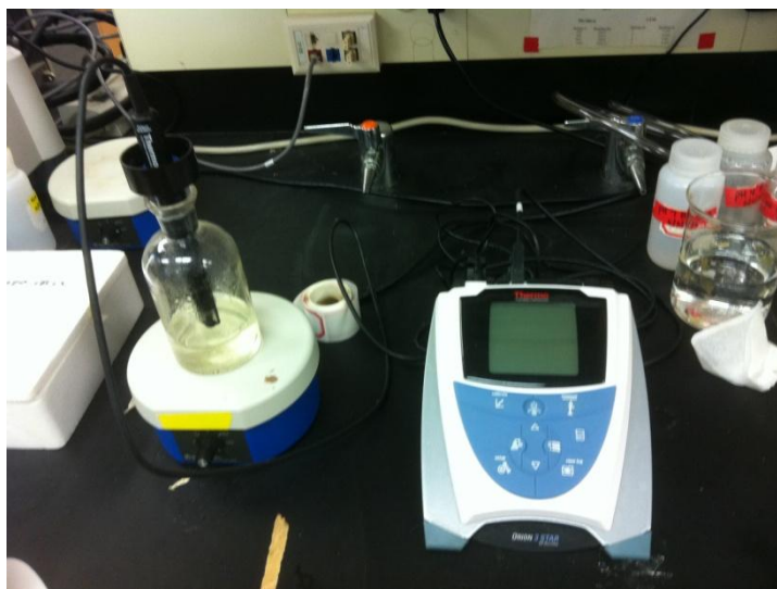
Figure 39: DO Meter (Dissolved Oxygen Test)
