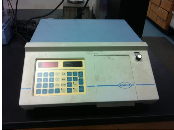
Figure 37: Hach DR/3000 Color Spectrometer (Total Phosphorus and Ammonia Test)
