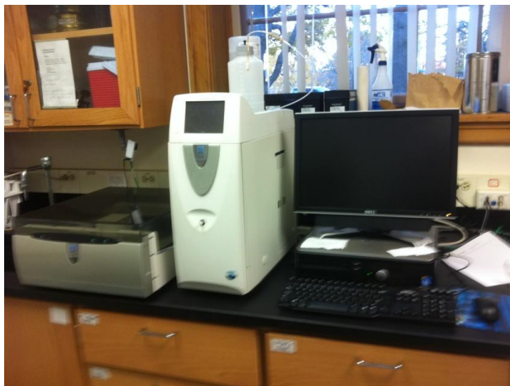
Figure 44: Ion Chromatography Set (Dissolved Ions Test)
