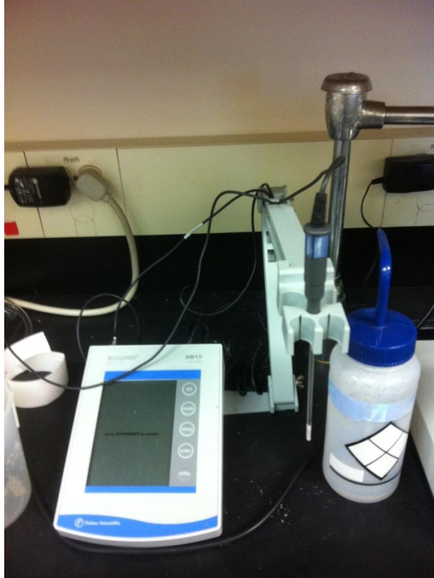
Figure 45: pH meter (pH Values Test)
