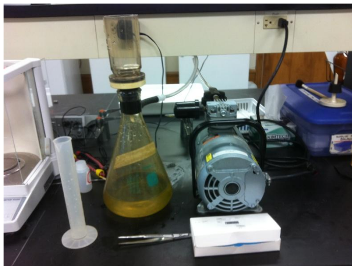
Figure 40: Vacuum, Graduate Cylinder, Filter, Tweezers (Total Suspended Solid Test)
