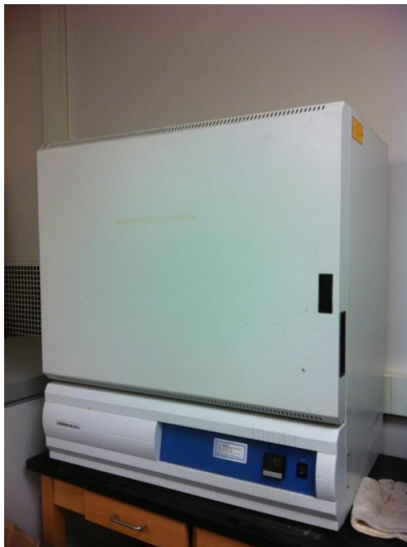
Figure 41: Dryer Machine (Total Suspended Solid Test)
