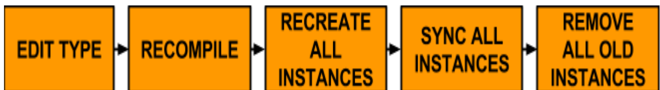
FIGURE 6.1. A process diagram showing the stages of syncing all instances to their modified type.
