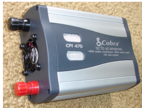
Figure 28: Example of a modified sine wave inverter (Zuzu, 2008)
