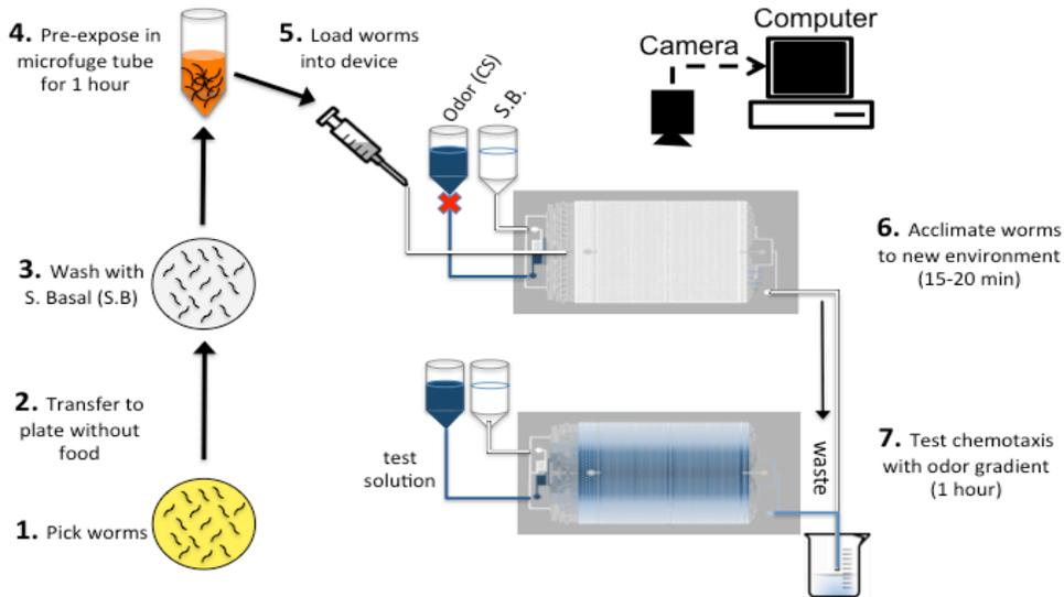
**D Pre-exposure and test within microfluidic device**
