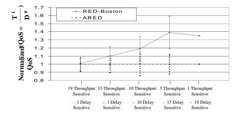
Figure 4.8: Simulation Set-1: Normalized QoS for Throughput-Sensitive Flows
