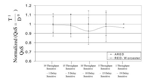
Figure 3.9: Normalized QoS for Throughput-Sensitive Flows
