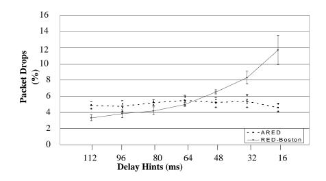
Figure 4.12: Simulation Set-2: Average Per Flow Percentage of Packets Dropped
