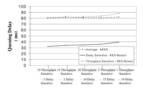
Figure 4.5: Simulation Set-1: Queuing Delays
