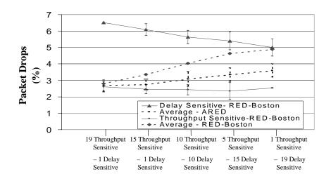
Figure 4.6: Simulation Set-1: Average Per Flow Percent of Packets Dropped
