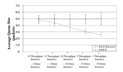
Figure 4.4: Simulation Set-1: Average Queue Size
