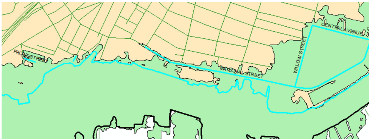
Figure 18. Map illustrating the flooding effects of a ten year flood under the conditions of the year 2050 on the Marginal Street area
