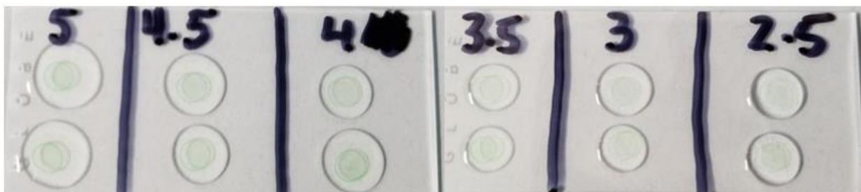
Figure 24: Testing setup for PDMS stamp with nanoparticles testing. Nanoparticle solution was dropped on the slide and then PDMS was cured over the dried drop.
