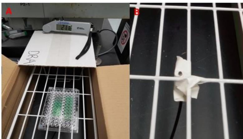
Figure 61: The fiber optic cable fixed in place under a metal grate and the well plate was moved to the cable for each trial. The fiber optic cable is attached to the grates of the stand using a custom prototyped holder and adhesive tape. The temperature is monitored within the enclosure using a standard thermoprobe.
