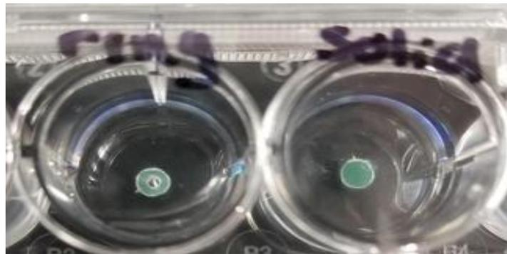
Figure 19: Preliminary foil testing with solid foil and ring foil, foils were bonded to polystyrene well plate using PDMS. The foils were cut using standard biopsy punches and then set in the PDMS. The PDMS was allowed to cure for 48 hours at room temperature.
