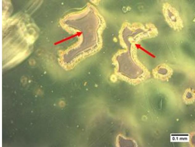
Figure 52: Specimen illustrating voids commonly seen in pressed samples as a result of nanoparticle clumping during drying of the solution. To improve the current fabrication technique, the process should be reevaluated and replicated with the goal of lessening and removing these voids.
