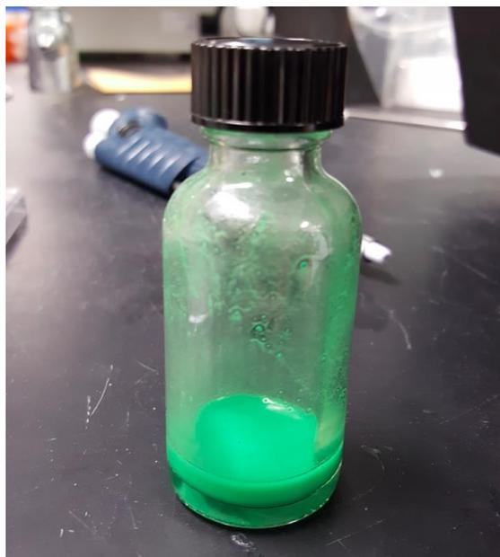
Figure 58: The hydrophilic form of the dye-based indicator. This dye was prepared using a combination of 200 proof ethanol and DI water in a 9:1 ratio.
