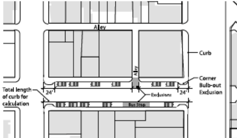
Figure 14: Diagram of a Street That Includes Bulb-outs
