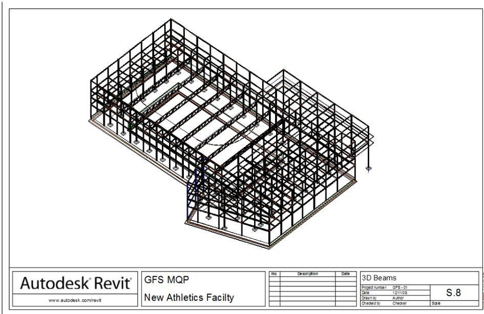
Figure 29: MQP Revit Model, Structural Beams 12/11/08
