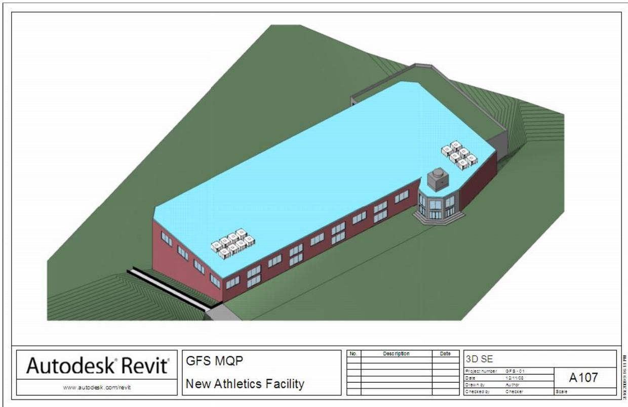
Figure 44: Solar Panel Roof Space (Highlighted in blue)
