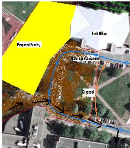
Figure 15: Demolition of the quad with normal traffic flow (blue) and changes (orange)
