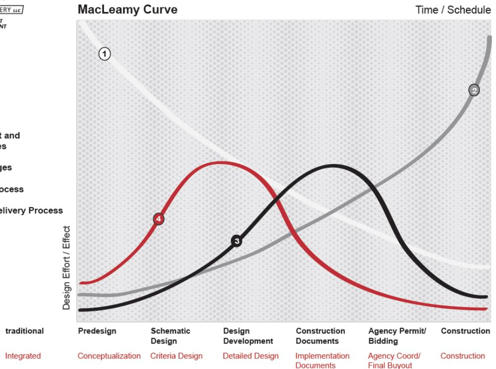
*Introduced in the Construction Users Roundtable's "Collaboration, Integrated Information, and the Project Lifecycle in Building Design and Construction and Operation" (WP-1202, August, 2004)", the "MacLeamy Curve" illustrates the advantages of Integrated Project Delivery.*
