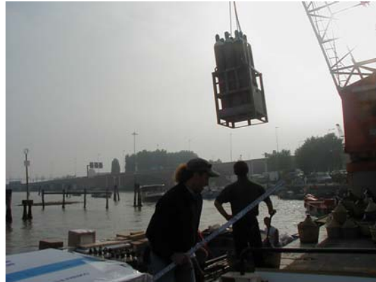
Figure 2: Unit Load Being Moved by Crane
