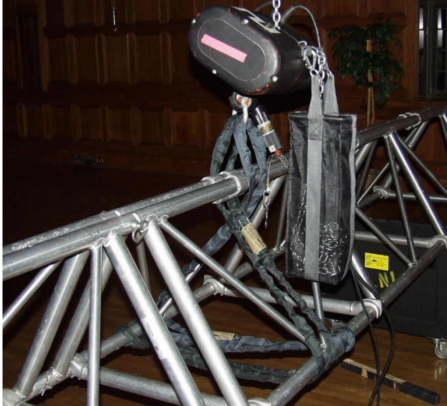
Figure 6: Sling wrapped around truss
