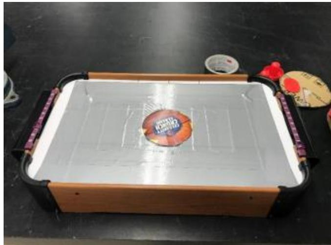
*Figure 38: Air Bearing Platform from an air hockey table (A. Brown et al., 2021)*
