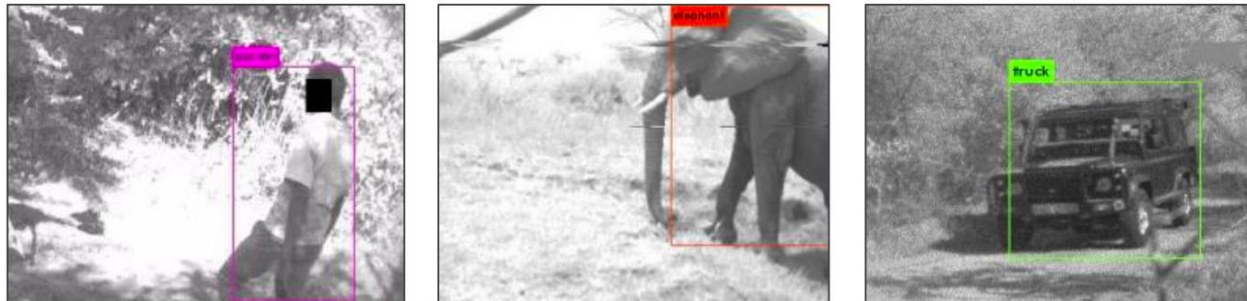
Figure 16: Example Screenshots of the Algorithm Spotting a Human (left), an Elephant (center), and a Vehicle (right)
