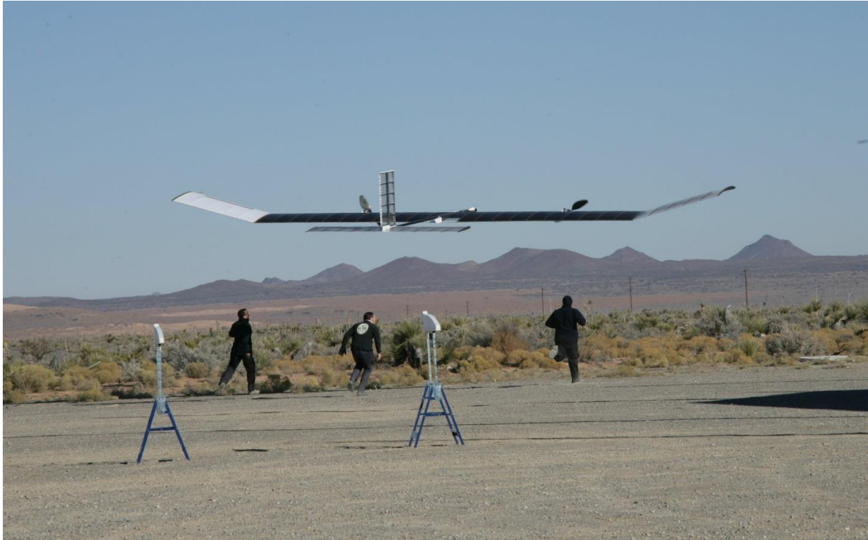
Figure 22: A Zephyr S Launch
