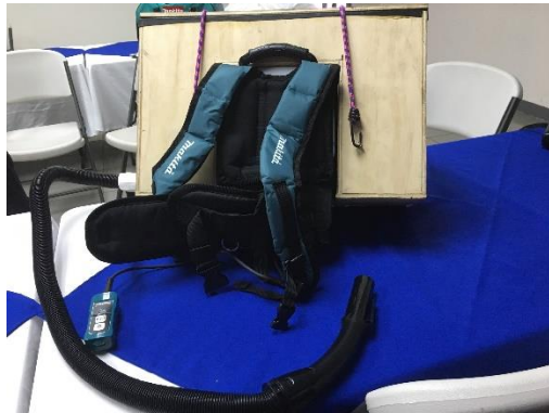
Figure 18: Custom backpack bee vacuum from Bomberos station in Belén, Costa Rica. February 21, 2020.
