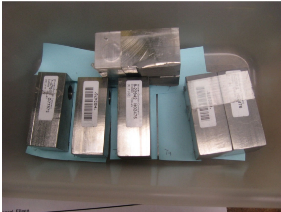
Figure 4: Ti-6Al-4V 2" x 1" x 1" test samples
